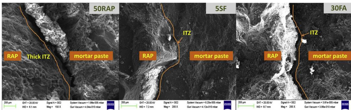
Fig. 5. Fe-SEM images showing ITZ of stated RAP-RCCP mixes.
