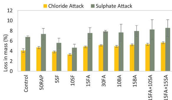
Fig. 12. Effect of SCMs after exposure to acid attack.
