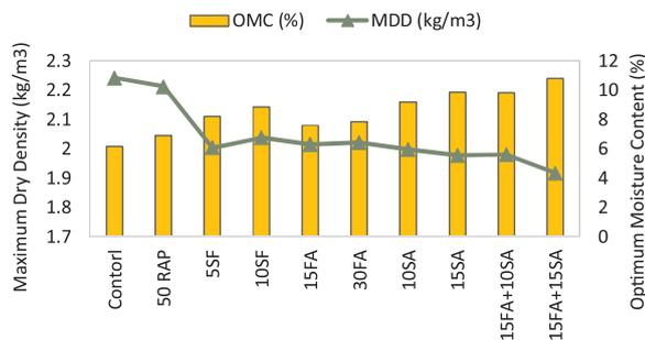
Fig. 3. Fresh properties of stated RCCP mixes.
