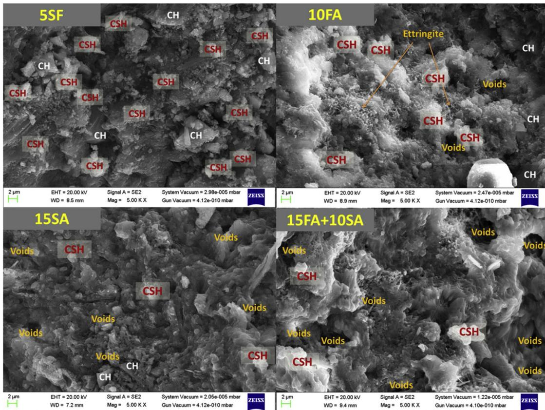
Fig. 9. Microstructure of stated RCCP mixes obtained using Fe-SEM.
