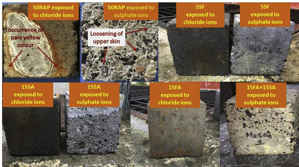
Fig. 13. Test specimens after being exposed to chloride & sulphate ions.
