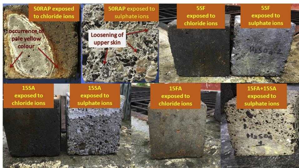
Fig. 13. Test specimens after being exposed to chloride & sulphate ions.
