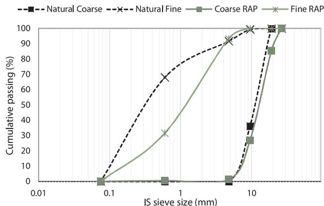
Fig. 2. Grain size distribution of aggregates.
