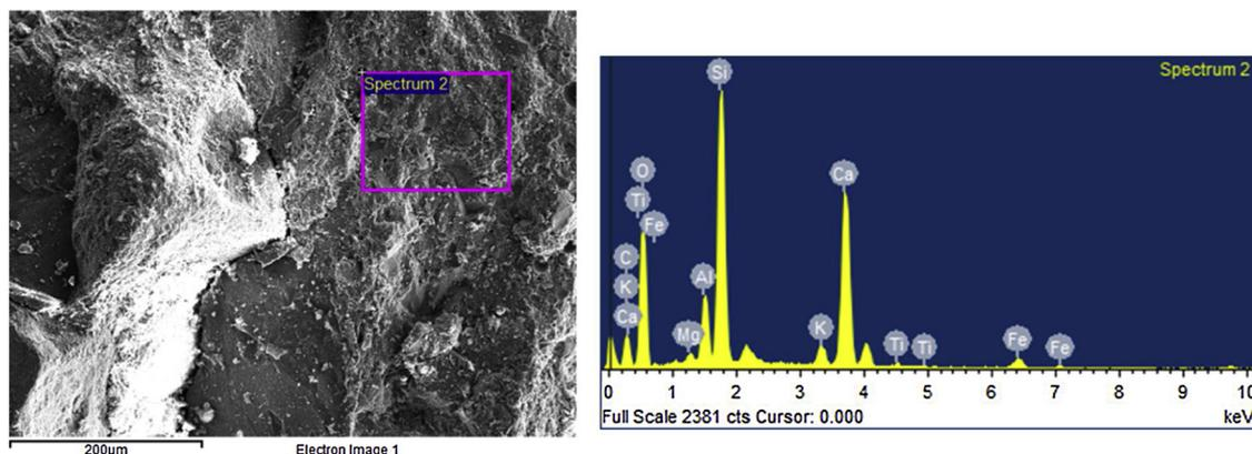
Fig. 11. EDX pattern of 50RAP mix containing 5% silica fume.
