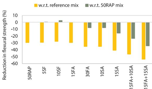
Fig. 7. Percentage reduction in the Modulus of Rupture.
