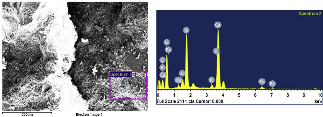
Fig. 10. EDX pattern of 50RAP mix containing 10% Fly Ash.
