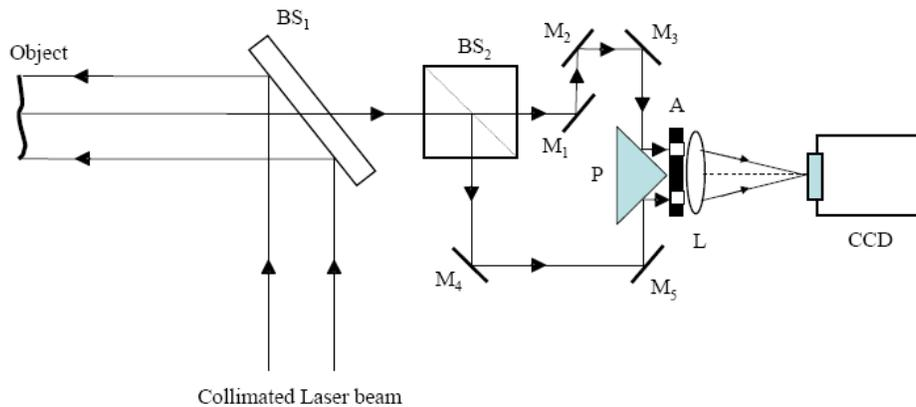
Fig. 2. Schematic of an in-plane insensitive digital shearography arrangement: O, Diffusely reflecting surface;  $BS_1$ , Beam splitter;  $BS_2$ , Cube beam splitter;  $M_1$ - $M_5$ , Mirrors; P, Front surfaces coated right angle prism; A, Two-aperture mask; L, Lens.
