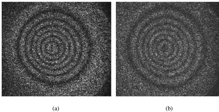
Fig. 4. Speckle correlation fringes with spatial phase shift: (a)  $-90^\circ$  and (b)  $0^\circ$
