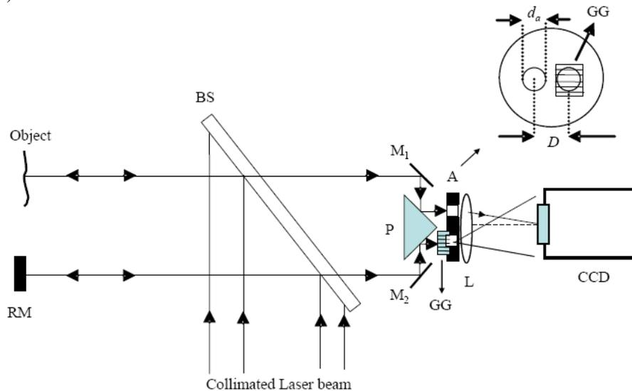
Fig. 1. Schematic of an out-of-plane sensitive digital speckle pattern interferometry arrangement: O, Object; RM, Reference mirror; BS, Beam splitter; M, Mirrors; P, Front surfaces coated right angle prism; A, double-aperture mask; GG, Ground glass; L, Imaging Lens.
