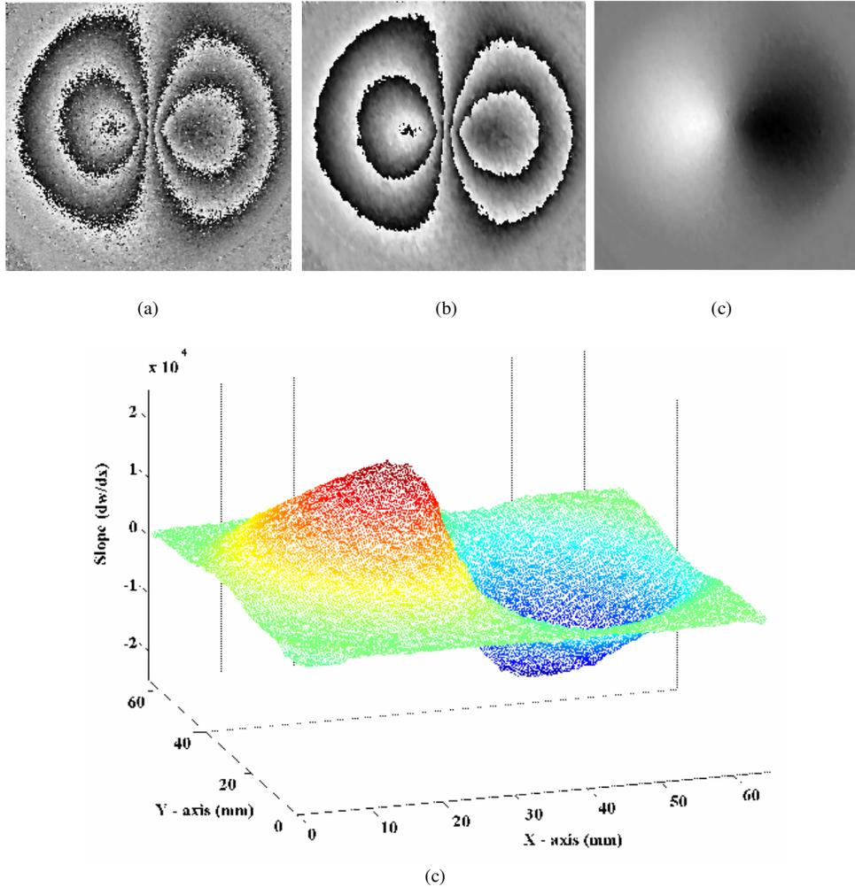
Fig. 6. Slope measurement: (a) raw and (b) filtered phase maps, (c) unwrapped 2D and (d) 3D plots
