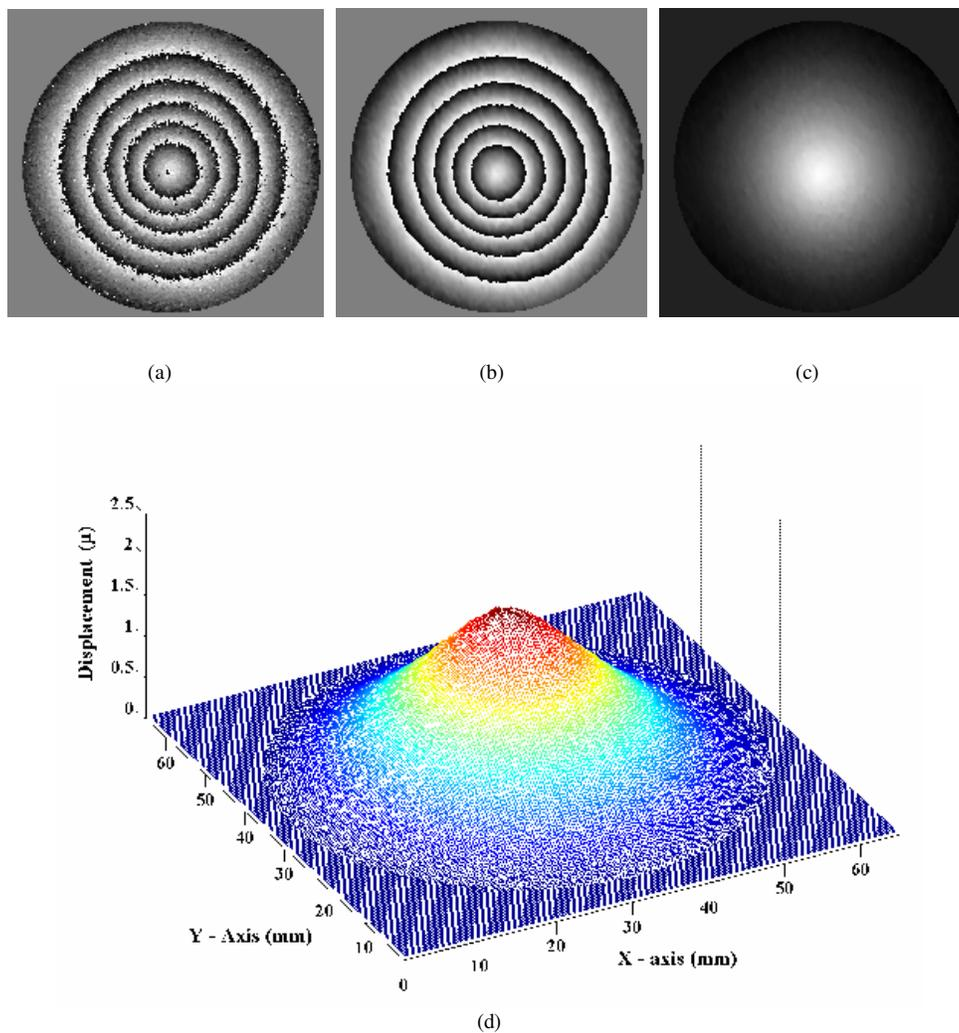
Fig. 5. Out-of-plane displacement measurement: (a) raw and (b) filtered phase maps, (c) unwrapped 2D and (d) 3D plots
