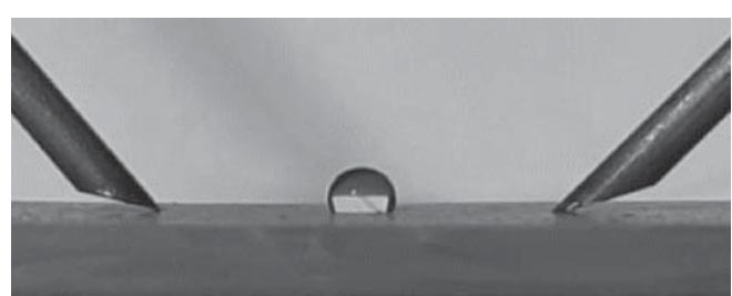
Figure 3 Test electrode arrangement
