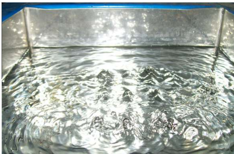
Fig. 4. Appearance of water surface when the 430 kHz was operational with 500 W power.
