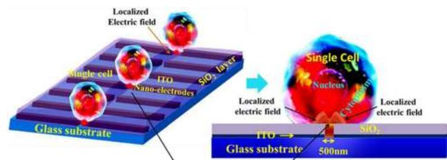
FIG. 1. Schematic representation of LSCNEP chip, where an intense electric field affects a small region of the cell membrane to permeate drug from outside to inside of the cell.
