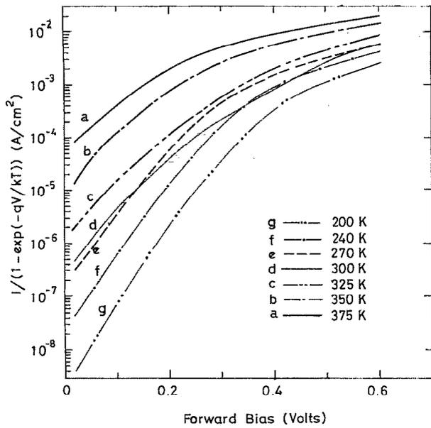
FIG. 4. Dark forward  $I$ - $V$  characteristics of ITO/ $p$ -InP junction with temperature as variable.
