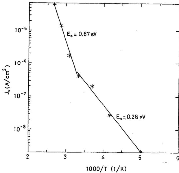
FIG. 6. Reverse saturation current plotted against inverse of temperature for ITO/p-InP junction.
