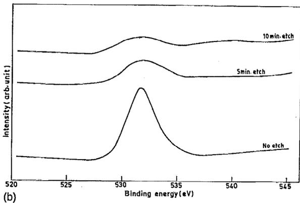
FIG. 1. (a) XPS In:3*d* spectra for ITO/*p*-InP junction at different argon ion etches. (b) XPS O:1*s* spectra for ITO/*p*-InP junction at different argon ion etches.
