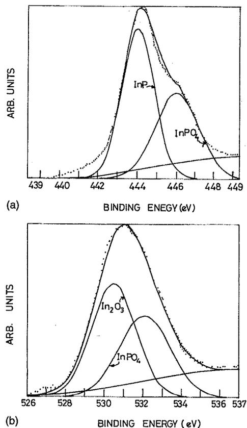
FIG. 2. (a) XPS In:3*d* spectra for 5 min argon ion etch of thin ITO/*p*-InP. Deconvoluted peaks correspond to In<sub>2</sub>O<sub>3</sub> and InPO<sub>4</sub>. Linear background is also shown. (b) XPS O:1*s* spectra for 5 min argon ion etch of thin ITO/*p*-InP. Deconvoluted peaks correspond to In<sub>2</sub>O<sub>3</sub> and InPO<sub>4</sub>. Linear background is also shown.
