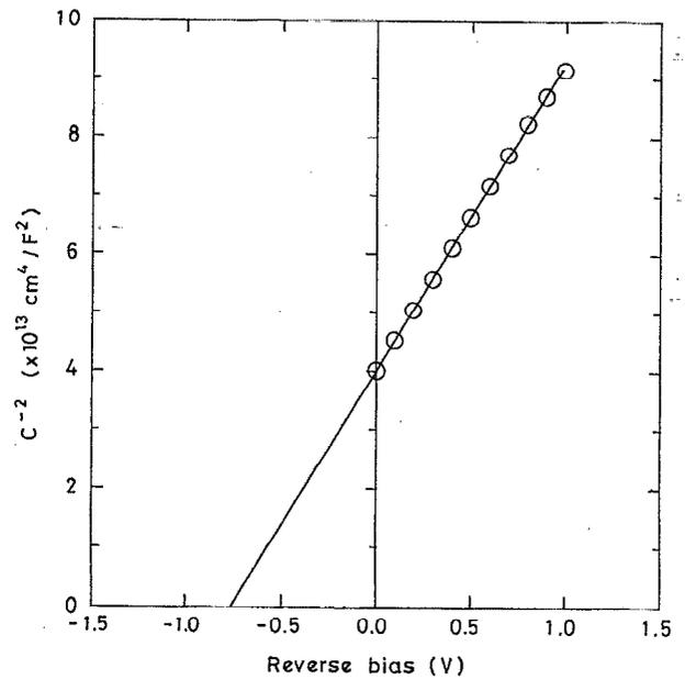
FIG. 7.  $1/C^2$  vs reverse bias voltage plot for ITO/p-InP junction.
