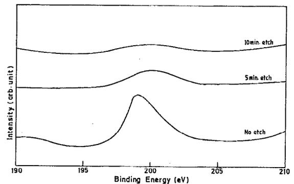
FIG. 3. XPS Cl:2*p* spectra for ITO/*p*-InP junction at different argon ion etches.
