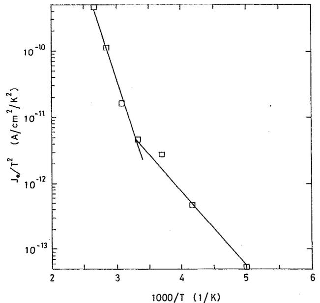
FIG. 5. Richardson plot for ITO/ $p$ -InP junction.
