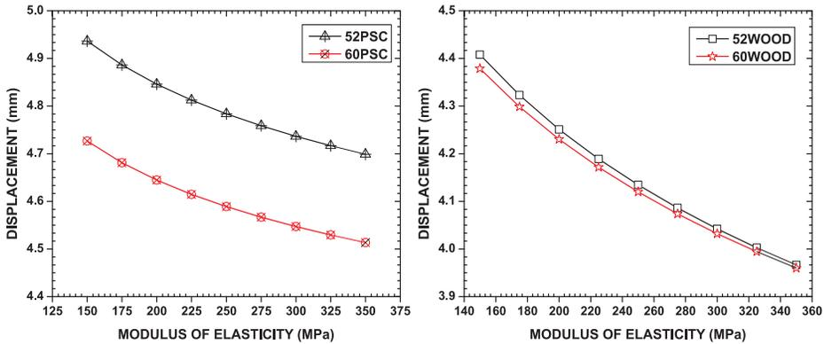
Figure 8. Displacement plots for both track models due to variation in ballast modulus: PSC (left) and WOOD (right).
