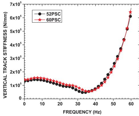
Figure 16. Track Stiffness of PSC track system.
