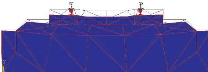
Figure 13. Displacement pattern for the track system due to subgrade with low stiffness.
