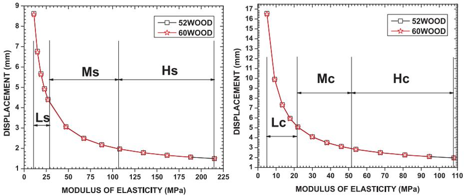
Figure 7. Displacement plots for wooden track model: sandy soil (left) and clayey soil (right).
