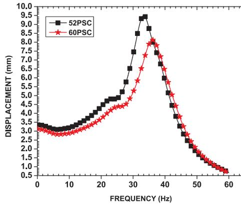
Figure 14. Vertical displacement of PSC track model.
