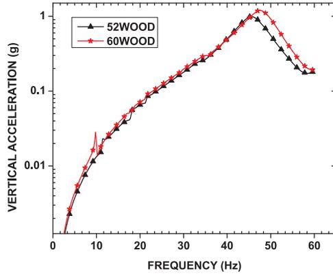
Figure 21. Vertical acceleration of wooden track system.
