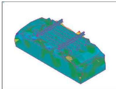
Figure 18. Mode shape (33.404 Hz) for 52 PSC track system.
