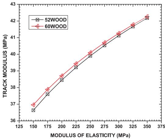
Figure 12. Track moduli for wooden track model due to variation in ballast modulus.
