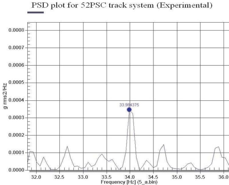
Figure 19. Power Spectral Density plot for 52PSC track system.
