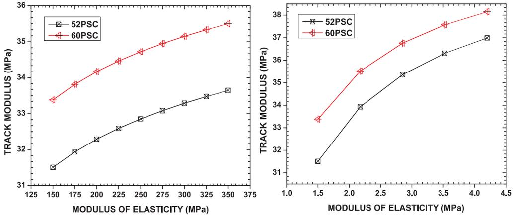
Figure 11. Track moduli for PSC track model due to variation in ballast (left) and rail pad modulus (right).
