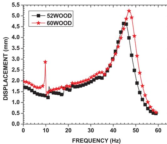
Figure 20. Vertical displacement of wooden track system.
