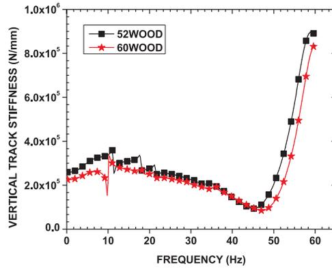
Figure 22. Track stiffness of wooden track system.
