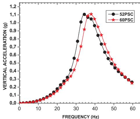
Figure 15. Vertical acceleration of PSC track model.
