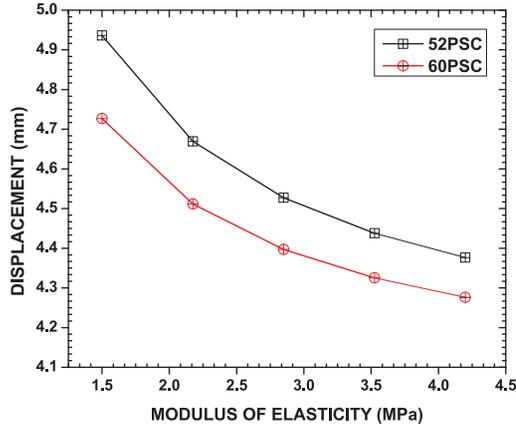
Figure 9. Displacement plots for both track models due to variation in rail pad modulus.
