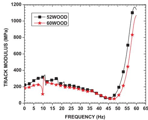
Figure 23. Track modulus of wooden track system.
