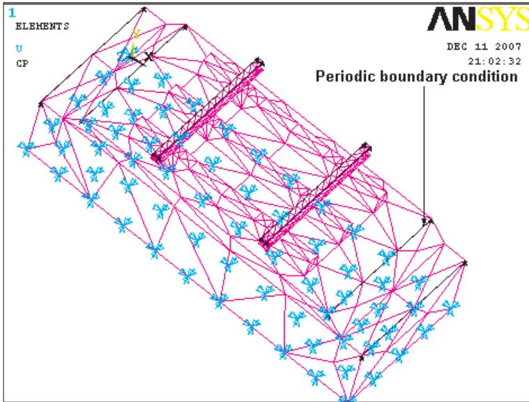
Figure 2. PSC sleeper track system with boundary conditions.
