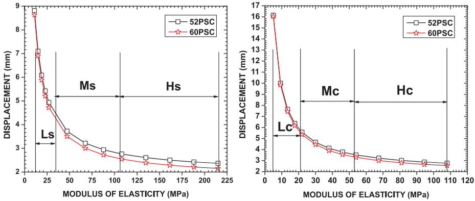
Figure 6. Displacement plots for PSC track model: sandy soil (left) and clayey soil (right).
