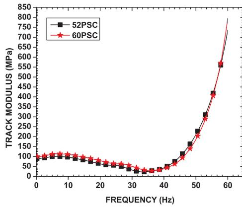
Figure 17. Track Modulus of PSC track system.
