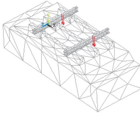
Figure 5. PSC sleeper track system with loading.
