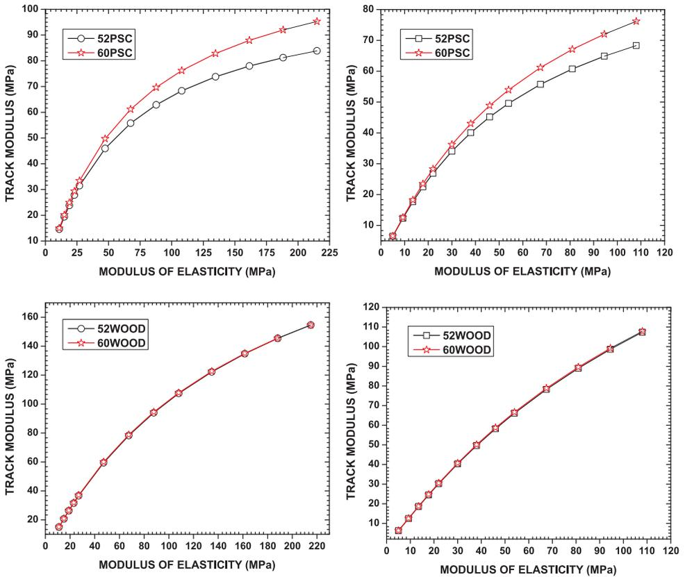
Figure 10. Track moduli due to variation in soil modulus: PSC track with sandy soil (top-left) and clayey soil (top-right); WOOD track with sandy soil (bottom-left) and clayey soil (bottom-right).
