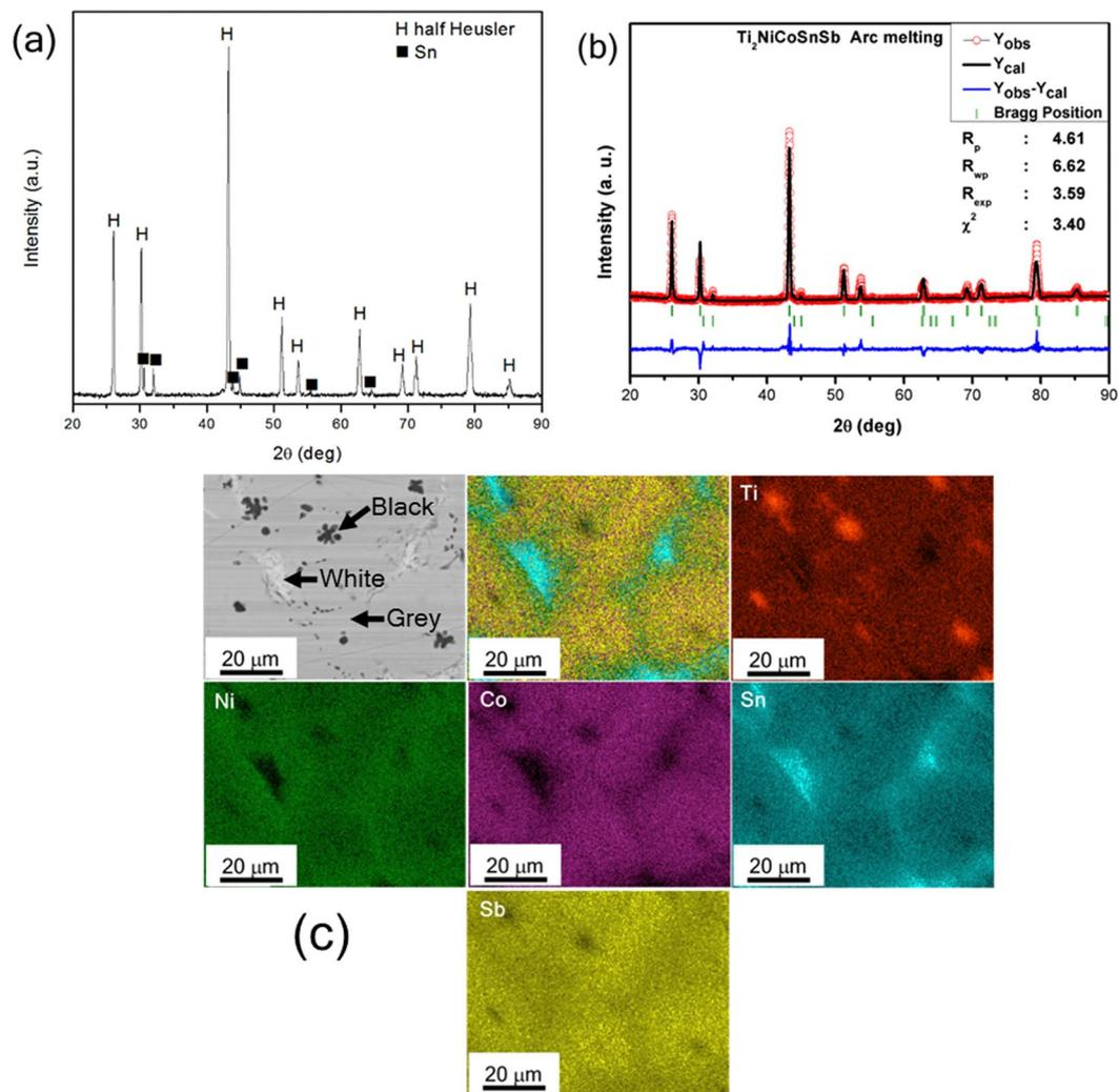
**Figure 1.** (a) XRD pattern, (b) Rietveld pattern of the VAM  $\text{Ti}_2\text{NiCoSnSb}$  alloy and (c) EDS Elemental mapping of the cast alloy confirming the presence of 3 phases.
