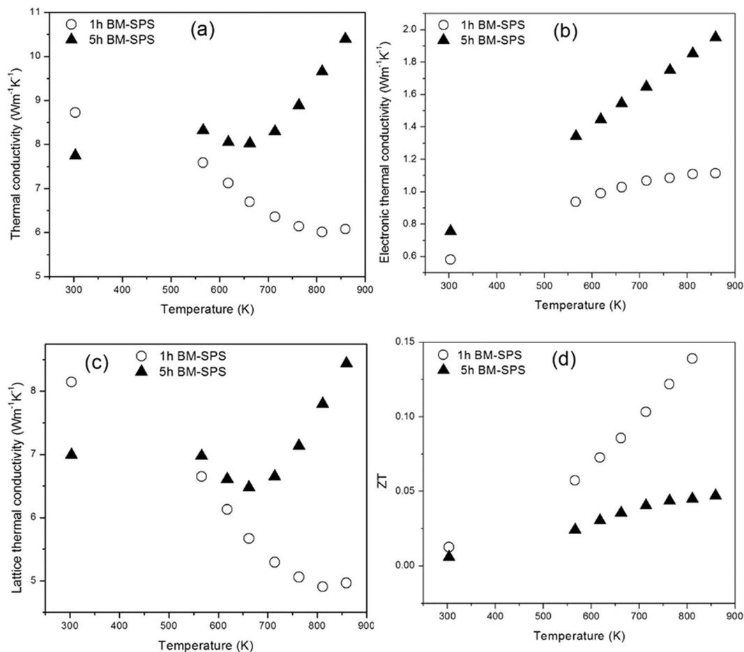
**Figure 5.** (a) Total thermal conductivity, (b) electronic thermal conductivity, (c) lattice thermal conductivity and (d) thermoelectric figure of merit (ZT) of Ti<sub>2</sub>NiCoSnSb alloy.
