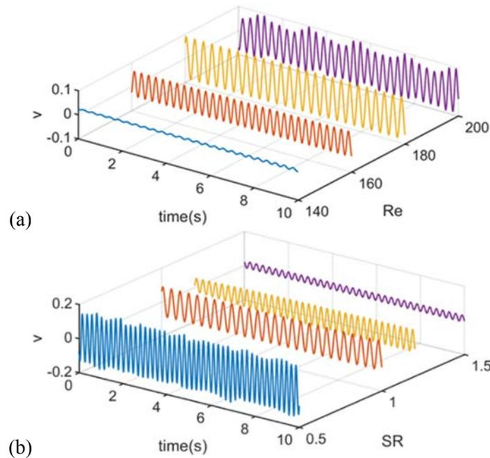
**Figure 6.** Time signals of transverse velocity component for different values of (a) Re and (b) SR.
