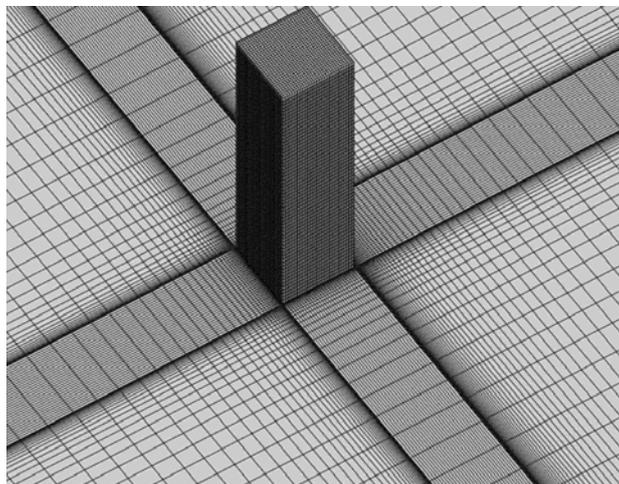
**Figure 2.** Grid distribution around the cylinder.
