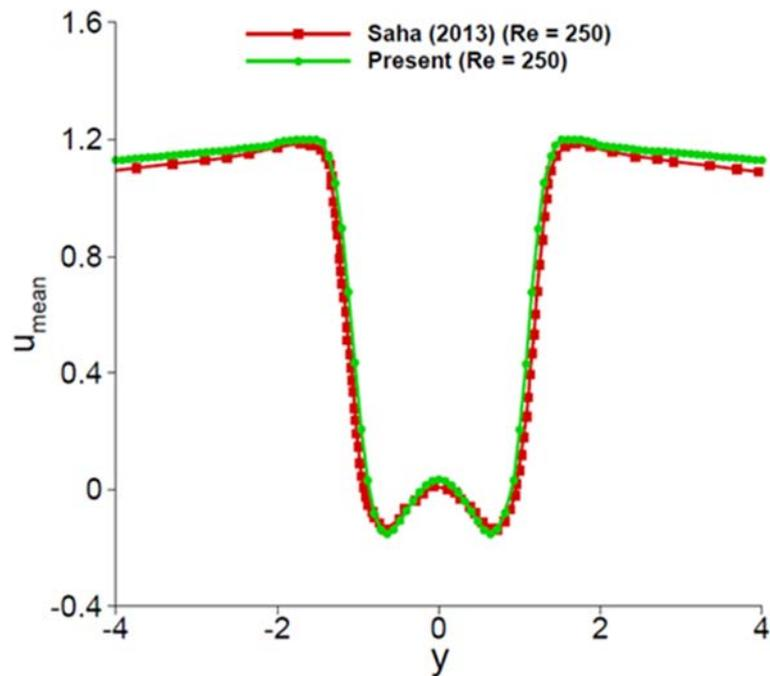
**Figure 3.** Variation of  $u_{mean}$  along transverse direction ( $y$ -direction) for  $AR = 3$  at  $x = 3$  and  $z = 2.5$ .
