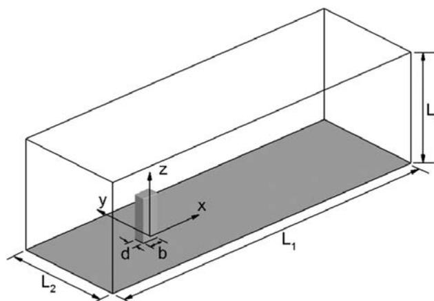
**Figure 1.** Schematic of three-dimensional computational domain.
