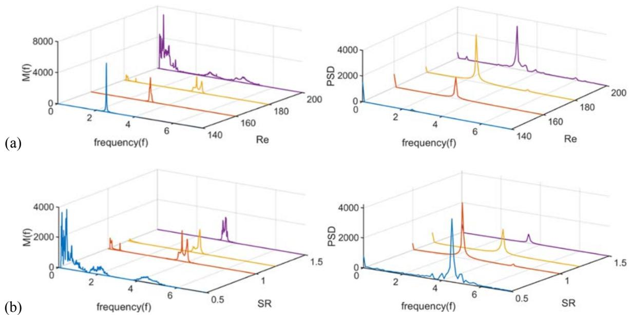
**Figure 9.** Marginal spectra (left) and Fourier spectra (right) for different values of (a) Re (b) SR.
