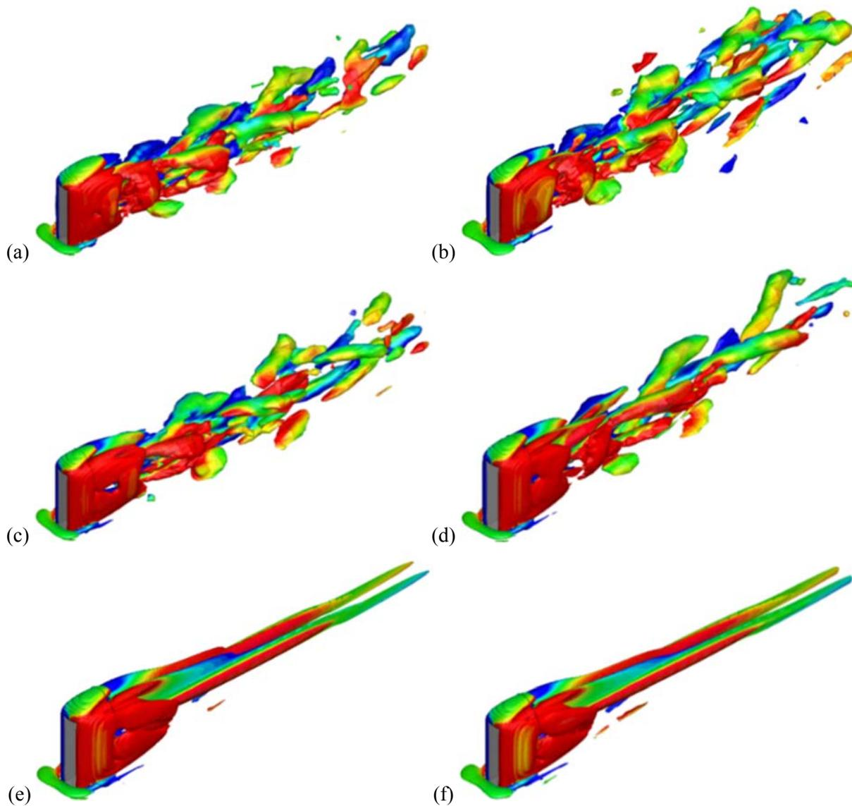
**Figure 5.** Instantaneous iso  $\lambda_2$ -surfaces, colored with z-vorticity, for  $Re = 180$  and different values of SR (a)  $SR = 0.5$  (b)  $SR = 1.0$  (c)  $SR = 1.2$  (d)  $SR = 1.5$  (e)  $SR = 1.8$  (f)  $SR = 2.0$ .
