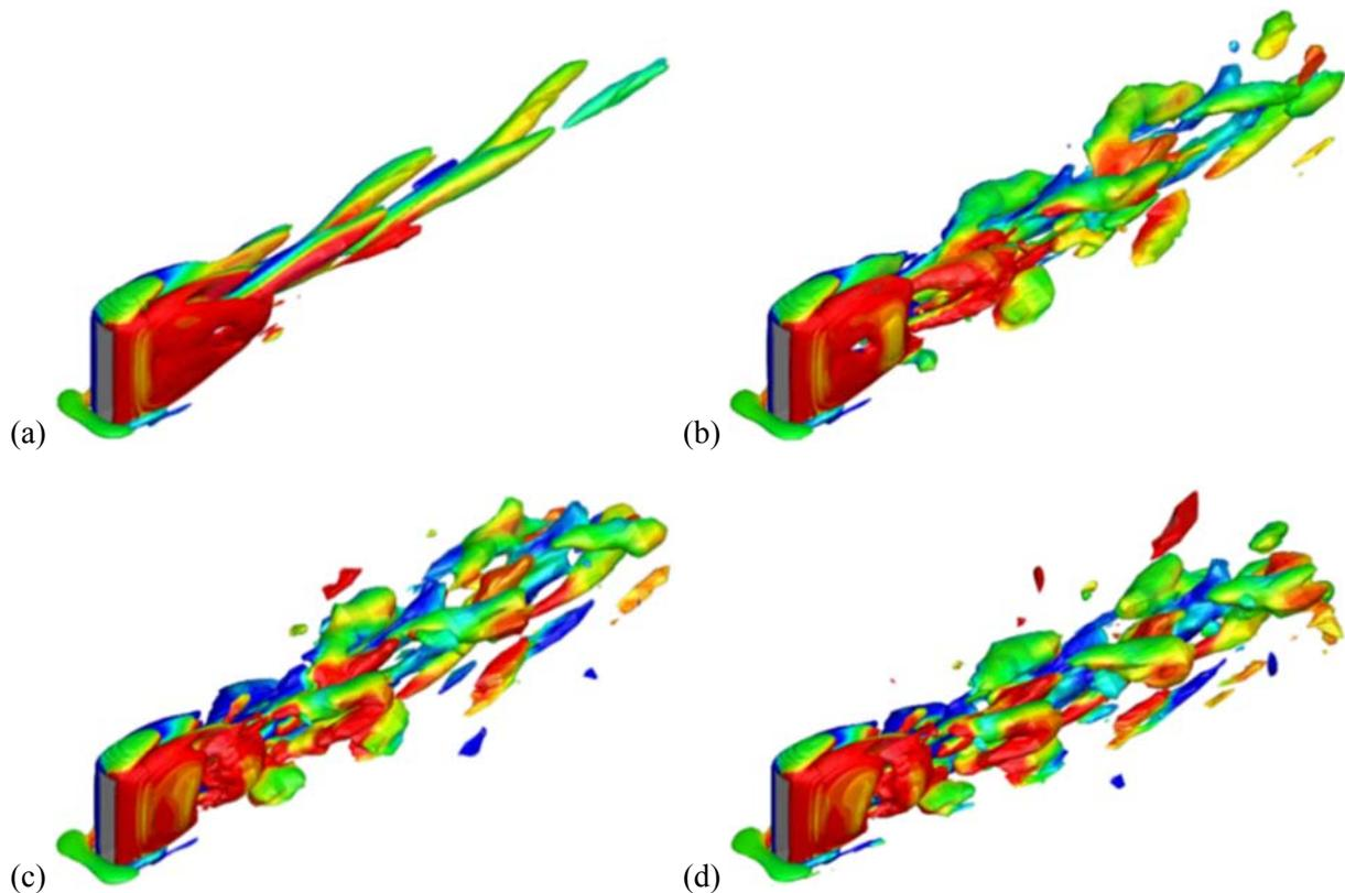
**Figure 4.** Instantaneous iso  $\lambda_2$ -surfaces, colored with  $z$ -vorticity, for  $SR = 1.0$  and different values of  $Re$  (a)  $Re = 140$  (b)  $Re = 160$  (c)  $Re = 180$  (d)  $Re = 200$ .
