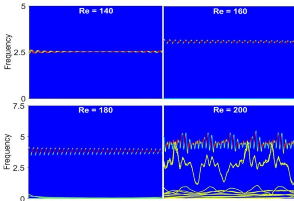
**Figure 7.** Hilbert spectra of transverse velocity signals for SR = 1.0 and different values of Re.
