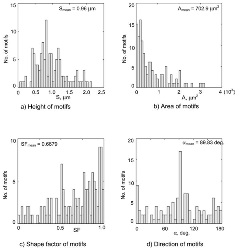
**Fig. 13** Histogram of motif parameters for ground surface: (a) height of motifs, (b) area of motifs, (c) shape factor of motifs, and (d) direction of motifs
