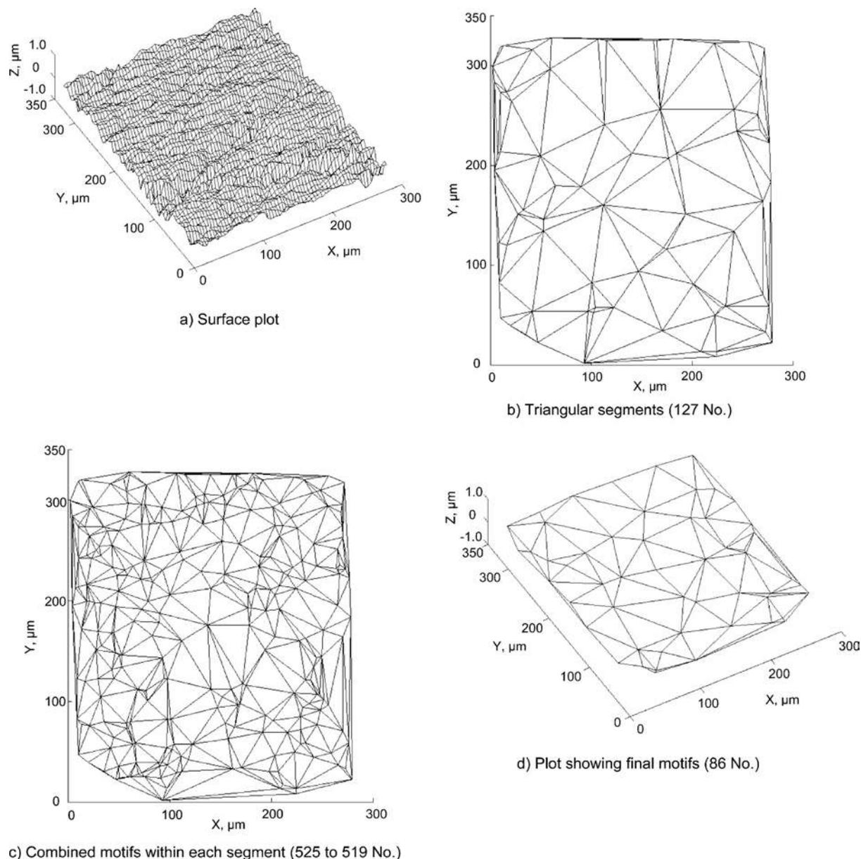
**Fig. 11** Stone-honed surface: (a) surface plot, (b) triangular segments (No. 127) (c) combined motifs within each segment (No. 525 to 519), and (d) plot showing final motifs (No. 86)
