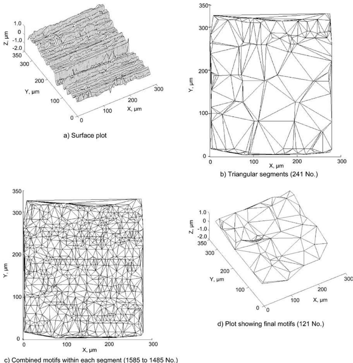
**Fig. 10** Ground surface: (a) surface plot, (b) triangular segments (No. 241), (c) combined motifs within each segment (No. 1585 to 1485), and (d) plot showing final motifs (No. 121)
