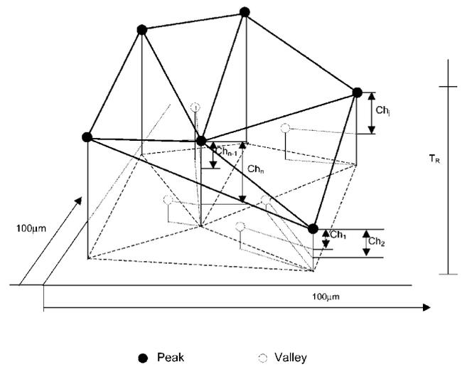
**Fig. 5** Relationship condition (Rule 4):  $[\min(CH_j) \leq 0.6T_R, j = 1, 2, \dots, n]$  or  $[\min(CH_j \leq 0.6 \max(CH_i), i = 1, 2, \dots, m; j = 1, 2, \dots, n)]$
