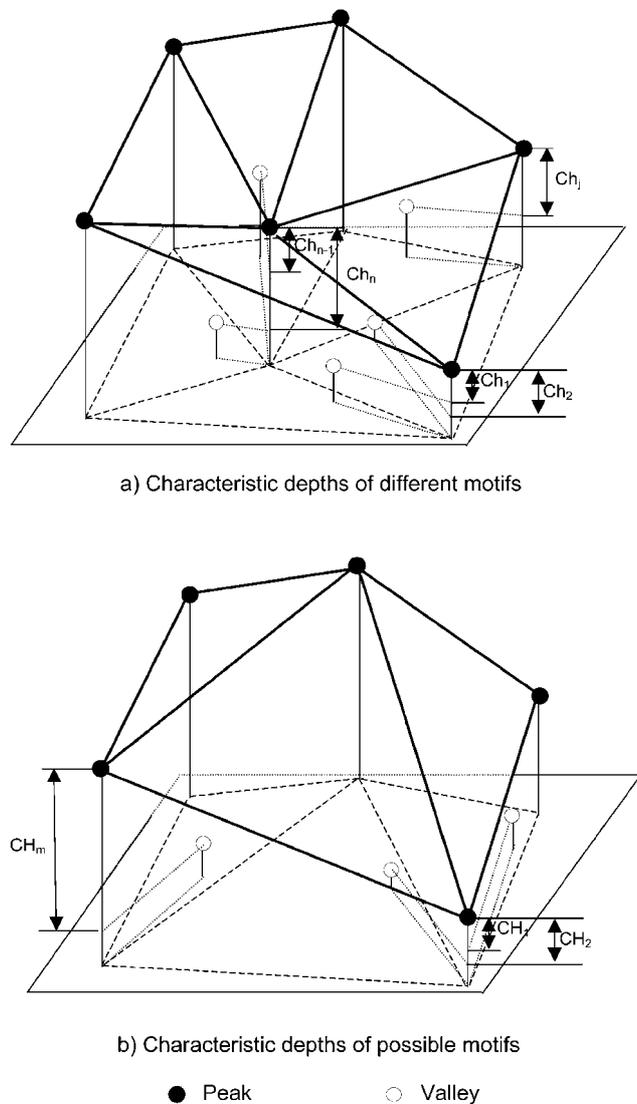
**Fig. 4** Magnification condition (Rule 3):  $[\max(CH_i) > \max(CH_j), i = 1, 2, \dots, m; j = 1, 2, \dots, n]$ . (a) Characteristic depths of different motifs and (b) characteristic depths of possible motifs
