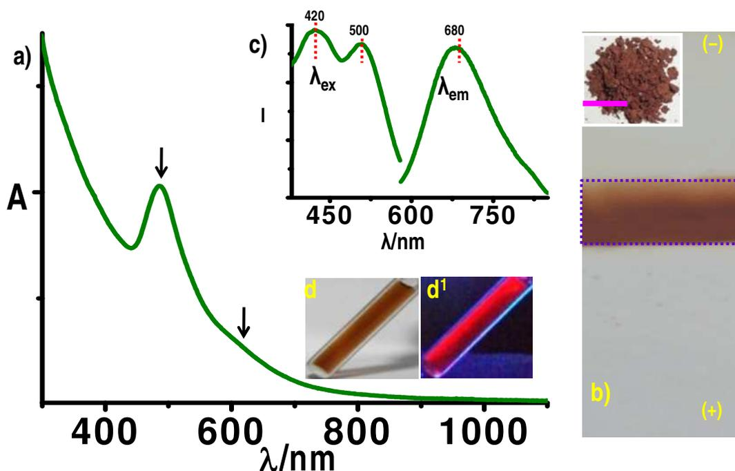
**Fig. 2** a) UV-vis absorption spectrum of the sample in (b). Distinct peaks are marked. b) Photograph of the PAGE band derived from aged crude. Inset of (b) is the aged crude cluster in powder form. Scale bars on inset of (b) is 1 cm. (c) Excitation and emission spectra of the same. Photographs of this solution in water collected under visible (d) and UV light (d<sup>1</sup>).
