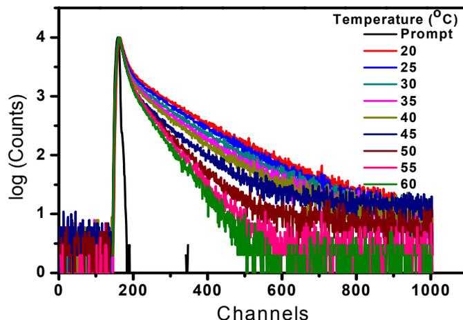
**Figure 6.** Fluorescence lifetime decay of ANS in GTHCC hydrogel {water: methanol (1:1)} with the variation in temperature; ( $\lambda_{\text{ex}} = 370 \text{ nm}$ ), [GTHCC] = 2 mg/mL, [ANS] = 4  $\mu\text{M}$ , (Channels=0.1 ns/chan.).
