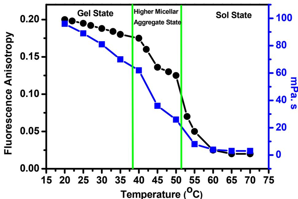
**Figure 5.** Plot for fluorescence anisotropy and microviscosity (mPa.s) of ANS in GTHCC hydrogel with variation of temperature, solvent taken water/methanol (1:1), ( $\lambda_{\text{ex}} = 380 \text{ nm}$ ), ([GTHCC] = 2 mg/mL). (Error = 3%)
