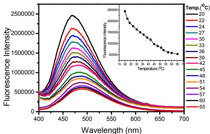
**Figure 3.** Plot of fluorescence Spectra of ANS in GTHCC hydrogel (water: methanol) with increase in temperature, ( $[ANS] = 4 \mu M$ , ( $\lambda_{ex} = 380 \text{ nm}$ ), Water: Methanol (1:1),  $[GTHCC] = 2 \text{ mg/mL}$ ).
