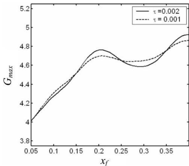
FIG. 7. Variation of maximum growth factor with heating element location for different values of time lag.  $L_w=2.0$  m,  $\lambda=0.0328$  W/m K,  $C_v=719$  J/kg K,  $\bar{\rho}=1.205$  kg/m<sup>3</sup>,  $c_0=401.2$  m/s,  $\bar{u}=0.5$  m/s, and  $T_w=1000$  K.
