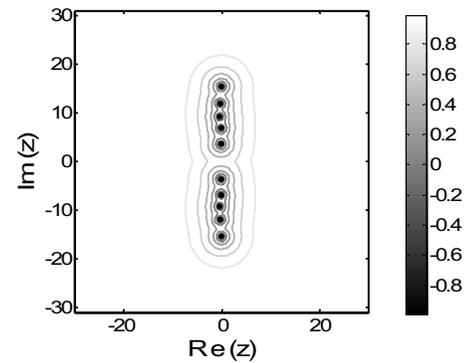
FIG. 9. Pseudospectra of a Rijke tube in which the heater is located at  $x_f = 0.18$ . The time lag was chosen as  $\tau = 0.1\pi$ .  $\lambda = 0.0328$  W/m K,  $C_v = 719$  J/kg K,  $c_0 = 399.6$  m/s,  $\bar{\rho} = 1.205$  kg/m<sup>3</sup>,  $L_w = 2.0$  m,  $T_w = 1000$  K, and  $\bar{u} = 0.5$  m/s.
