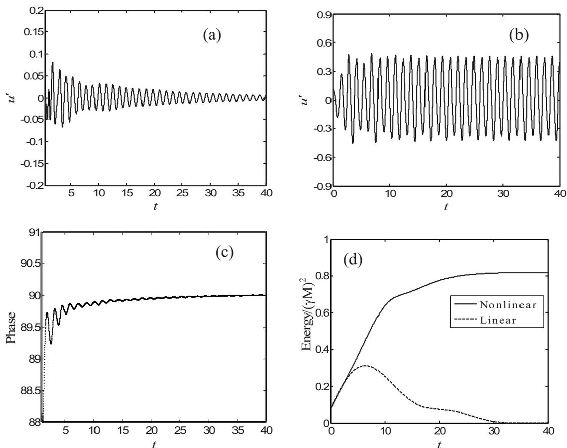
FIG. 4. Evolution of nondimensional acoustic velocity when the initial conditions are (a)  $\eta_1(0)=0.15$  and (b)  $\eta_1(0)=0.2$ ,  $x_f=0.29$ ,  $c_0=399.6$  m/s,  $L_w=3.6$  m,  $\bar{u}=0.5$  m/s,  $\bar{p}=1.205$  kg/m<sup>3</sup>,  $T_w=1000$  K,  $C_v=719$  J/kg K, and  $\lambda=0.0328$  W/m K. (c) Evolution of phase and (d) linear and nonlinear evolutions of the acoustic energy when the initial condition is  $\eta_1(0)=0.2$ .
