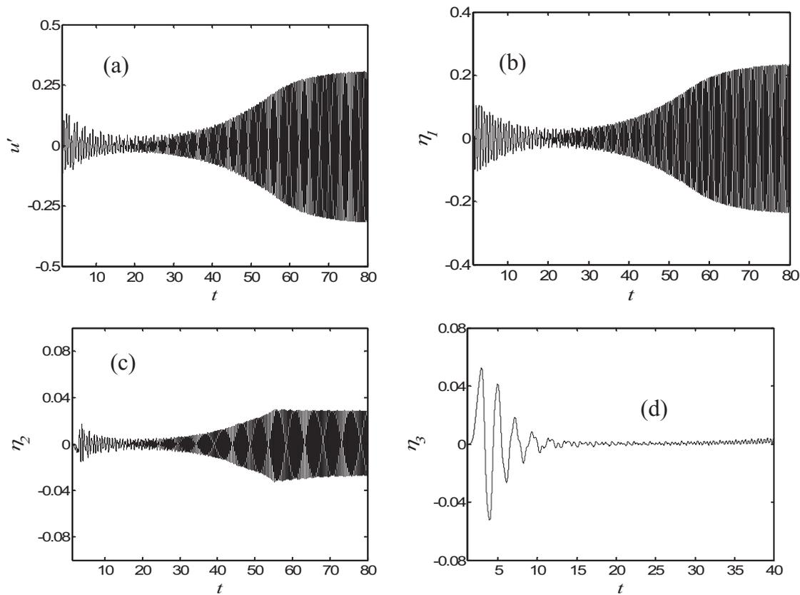
FIG. 5. (a) Nondimensional evolution of acoustic velocity when the initial condition is  $\eta_1(0)=0.18$ ; [(b)–(d)] evolution of the acoustic velocity projected onto the various Galerkin modes.  $L_w=3.6$  m,  $\lambda=0.0328$  W/m K,  $C_v=719$  J/kg K,  $\bar{\rho}=1.205$  kg/m<sup>3</sup>,  $\bar{u}=0.5$  m/s,  $T_w=1000$  K,  $\tau=0.45\pi$ ,  $x_f=0.29$ , and  $c_0=399.6$  m/s.
