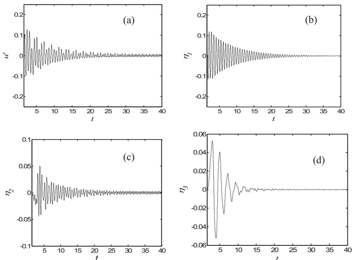
FIG. 6. (a) Linear evolution of acoustic velocity when the initial condition is  $\eta_1(0)=0.18$ ; [(b)–(d)] evolution of the acoustic velocity projected onto the various Galerkin modes. The conditions are the same as those of Fig. 5.
