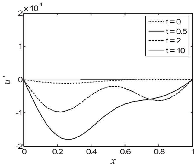
FIG. 8. Spatial variation of the acoustic velocity at various instants of time. The initial condition is chosen to be the optimum initial condition which yields the maximum growth factor.  $L_w=2.0$  m,  $\tau=0.1\pi$ ,  $\lambda=0.0328$  W/m K,  $C_v=719$  J/kg K,  $\bar{\rho}=1.205$  kg/m<sup>3</sup>,  $c_0=401.2$  m/s,  $\bar{u}=0.6$  m/s, and  $T_w=900$  K.
