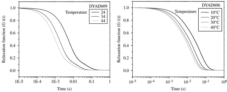
**Figure 2.** Relaxation function of a sound coat DYAD609 and DYAD606 viscoelastic material
