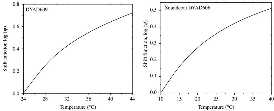
**Figure 3.** Shift function of a sound coat DYAD609 and DYAD606 viscoelastic material
