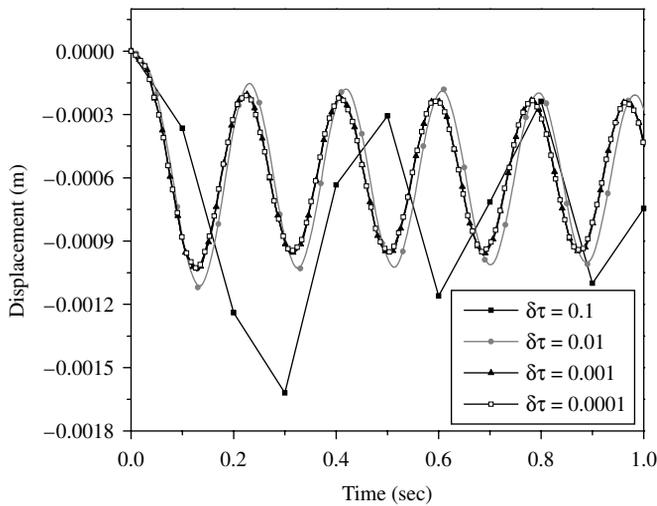
**Figure 4.** Transient response of sandwich beam at different time steps
