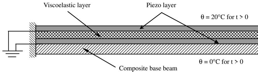
**Figure 1.** Schematic diagram of piezo-thermo-viscoelastic composite beam
