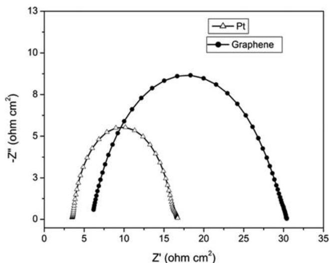
FIG. 6. Nyquist plots of graphene and Pt in a symmetric cell configuration showing a comparable electrochemical behavior.
