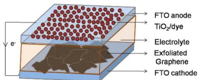
FIG. 1. (Color online) Schematic of thermally exfoliated graphene counter electrode based DSSC.
