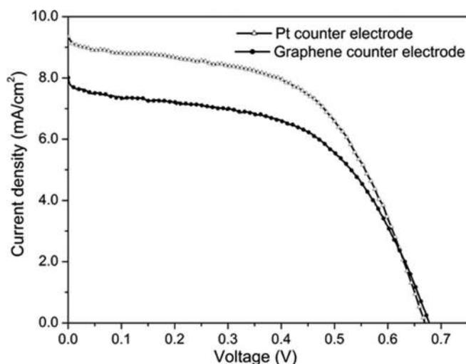
FIG. 7. Current voltage curves for graphene (EG) and Pt counter electrodes based DSSCs obtained using AM 1.5 solar illumination with an intensity of 1 sun.
