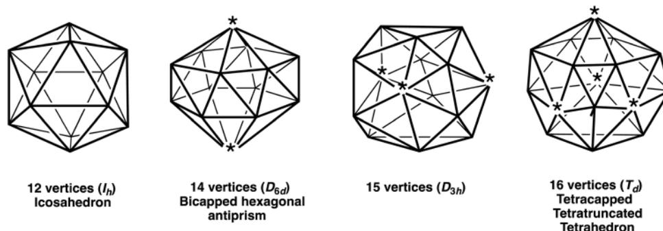
Fig. 2 The four Frank–Kasper deltahedra with the degree 6 vertices starred.
