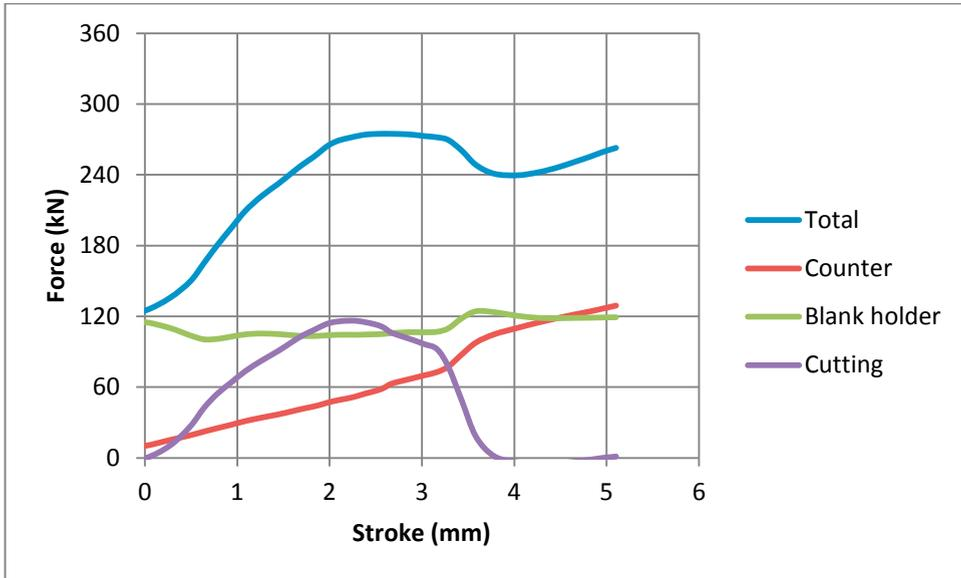
Fig. 2. Force-stroke diagram of fine blanking of AISI 304 Stainless Steel with rubber
