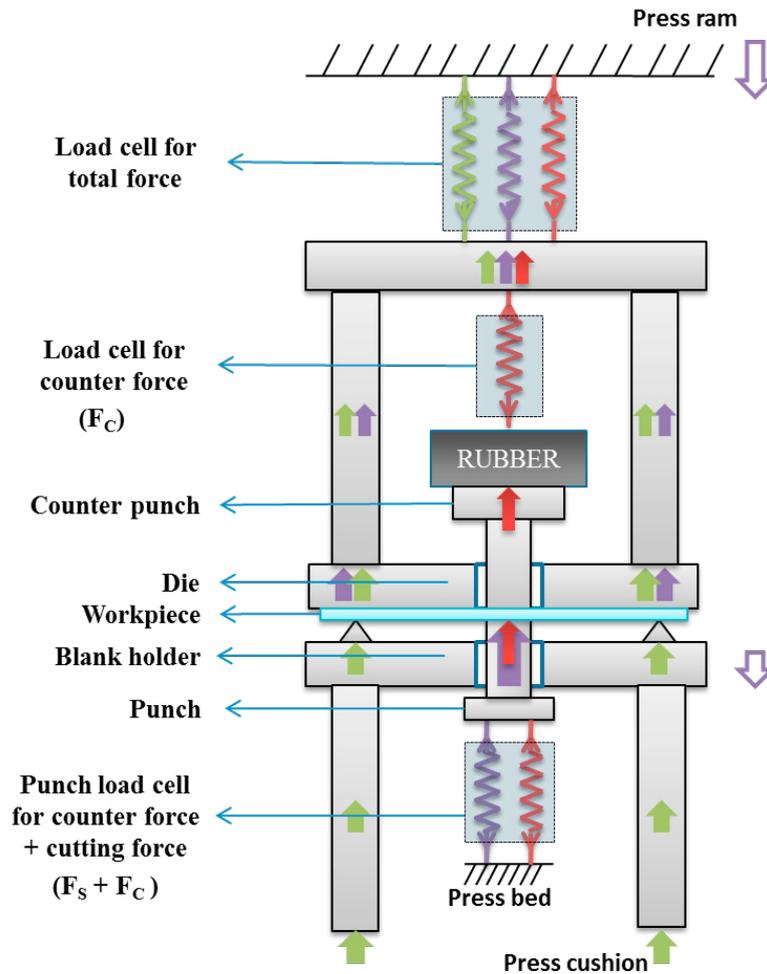
Fig. 1. Schematic – Fine blanking with rubber for counter force
