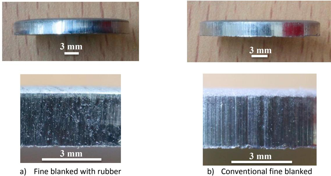
Fig. 4. Photographs of specimens showing the fine blanked edge
