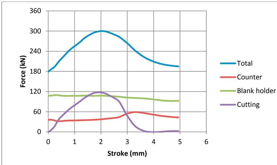
Fig. 3. Force-stroke diagram of conventional fine blanking of AISI 304 Stainless Steel
