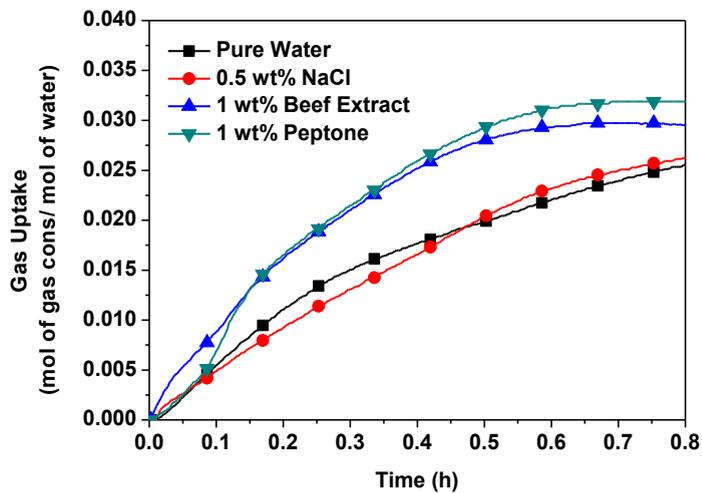
Fig. 2. Comparison of average gas uptake during methane hydrate formation individually with pure water, NaCl, Beef Extract and Peptone (the different components present in the Nutrient Broth).
