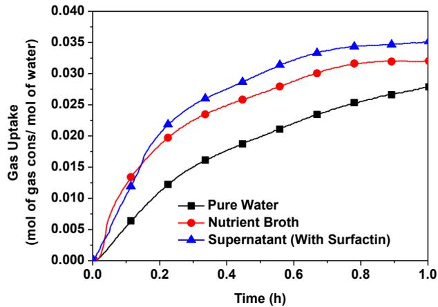
Fig. 1. Comparison of average gas uptake during methane hydrate formation from different hydrate forming solutions: pure water, nutrient broth and cell free Surfactin containing supernatant.
