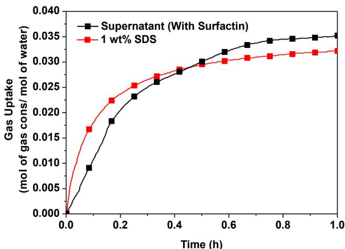
**Fig. 3. Comparison of average gas uptake during methane hydrate formation with cell free supernatant containing the biosurfactant Surfactin and with 1 wt% SDS.**
