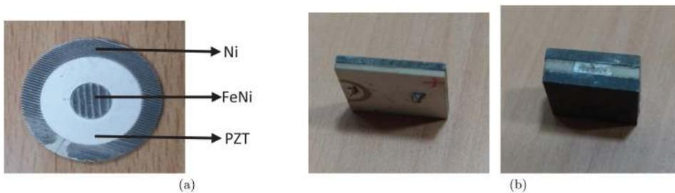
FIG. 2. (a) Fabricated epoxy-free ring composite. (b) Epoxy bonded bilayered and trilayered composite.
