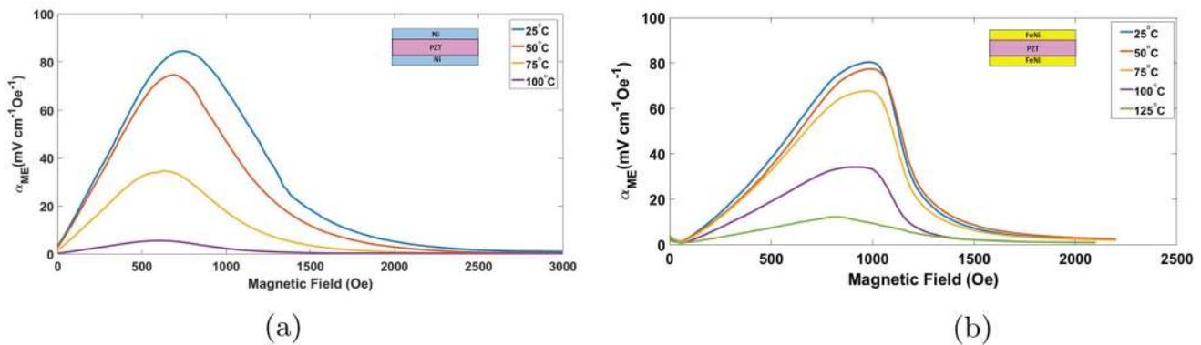
FIG. 9. (a)  $\alpha_{ME}$  for Ni/PZT/Ni trilayered epoxy bonded composite at different temperatures. (b)  $\alpha_{ME}$  for FeNi/PZT/FeNi trilayered epoxy bonded composite at different temperatures.
