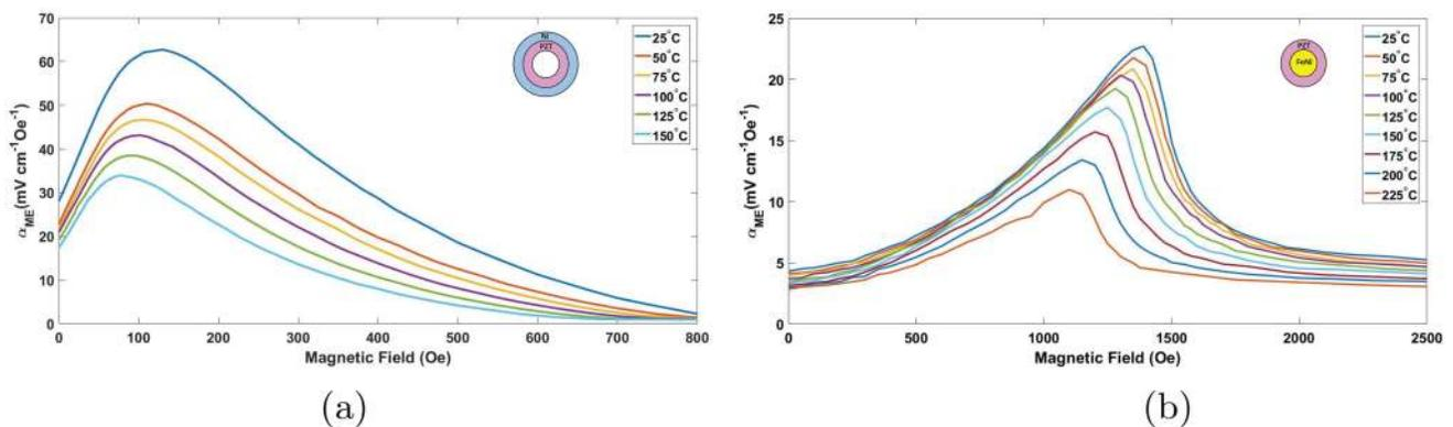
FIG. 10. (a)  $\alpha_{ME}$  for Ni/PZT epoxy-free ring composite at different temperatures. (b)  $\alpha_{ME}$  for FeNi/PZT epoxy-free ring composite at different temperatures.
