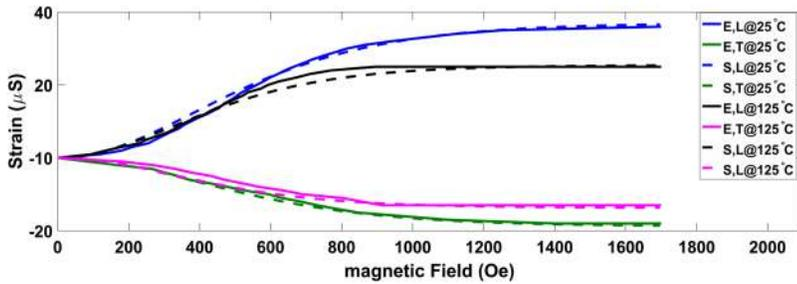
FIG. 6. Magnetostriction of nickel—experimental and simulation results at 25 °C and 125 °C. E: experimental; S: simulation; L: longitudinal; T: transverse.
