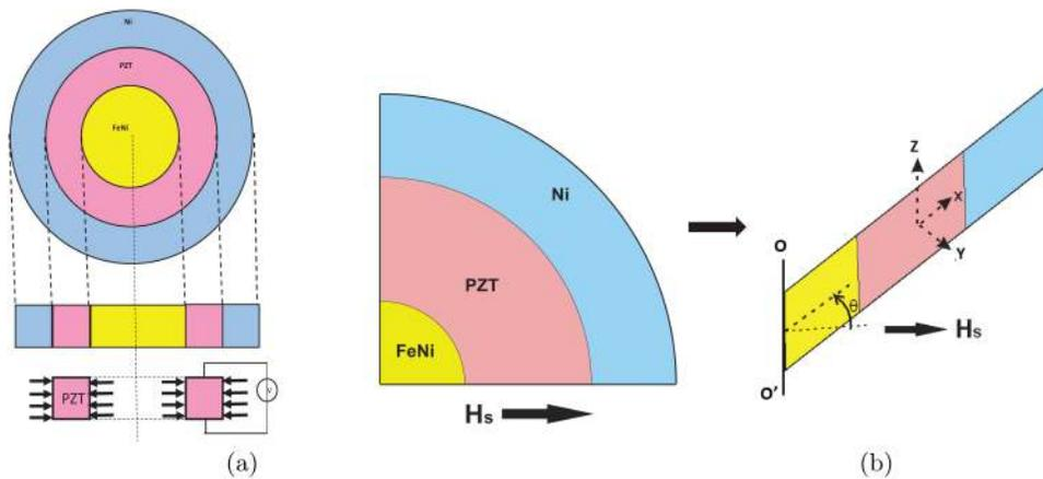
FIG. 4. (a) The schematic of the ring ME sample. (b) Schematic of the top view of a quadrant of the ring composite (since the four quadrants are symmetric); Schematic of a strip from the quadrant of the sample being subjected to magnetic field.
