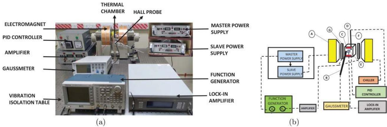
FIG. 3. (a) The experimental setup to measure ME coefficient. (b) Schematic of the experimental setup to measure ME coefficient. A: electromagnet, B: Hall probe, C: aluminum heater plate, D: thermal chamber, E: sample, F: thermocouple, G: Helmholtz coil.
