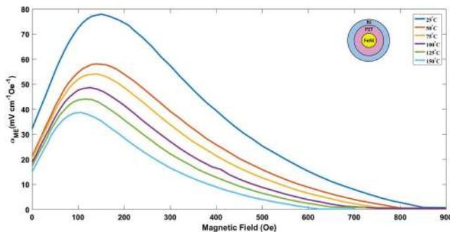
FIG. 7. Magneto-electric coefficient of FeNi/PZT/Ni ring composite at 25 °C, 50 °C, 75 °C, 100 °C, 125 °C, and 150 °C.
