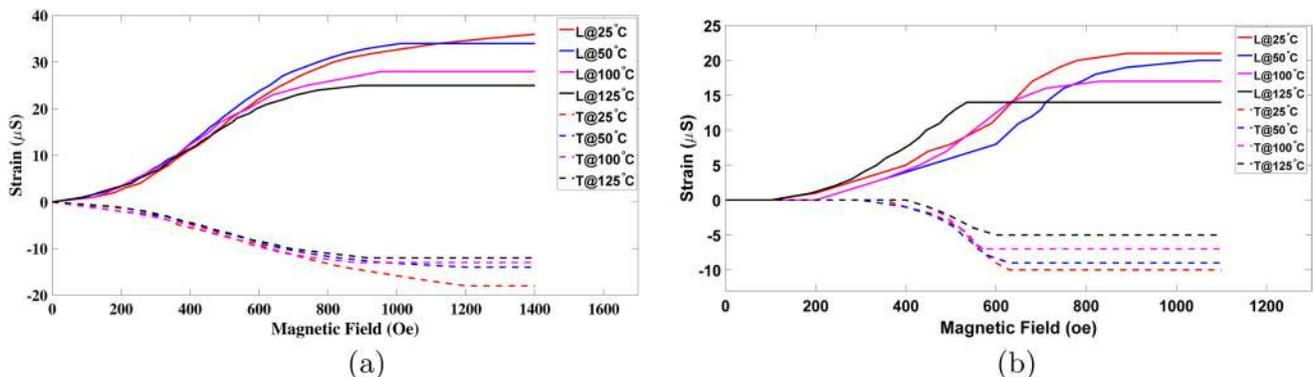
**FIG. 5.** (a) Magnetostriction of nickel—experimental results at 25 °C, 50 °C, 100 °C, and 125 °C. (b) Magnetostriction of FeNi—experimental results at 25 °C, 50 °C, 100 °C, and 125 °C (L: longitudinal; T: transverse).
