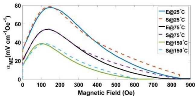
FIG. 13. Experiment vs simulation ME coefficient for the FeNi/PZT/Ni ring composite at  $25^\circ\text{C}$ ,  $75^\circ\text{C}$ , and  $150^\circ\text{C}$  (frequency of ac signal = 1 kHz). E: experiment; S: simulation.
