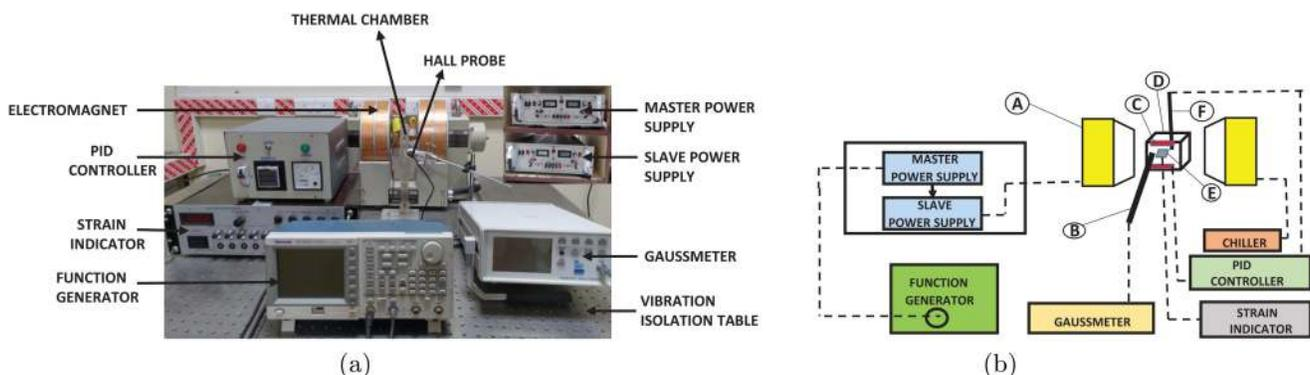
**FIG. 1.** (a) The experimental setup to measure magnetostriction. (b) Schematic of the experimental setup to measure magnetostriction. A: electromagnet, B: Hall probe, C: aluminum heater plate, D: thermal chamber, E: sample, F: thermocouple.
