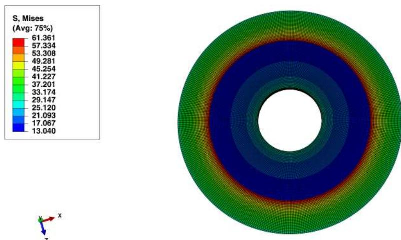
FIG. 12. ABAQUS results for the prestress developed at the Ni/PZT interface of the FeNi/PZT/Ni ring composite.
