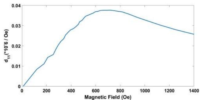
FIG. 8. Magnetic field dependence of piezomagnetic coefficient  $d_{11}$  for Ni at room temperature.
