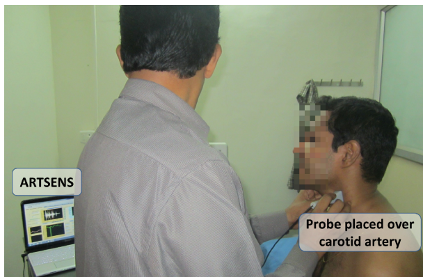
FIGURE 3. ARTSENS used to perform carotid artery stiffness measurement of a volunteer.
