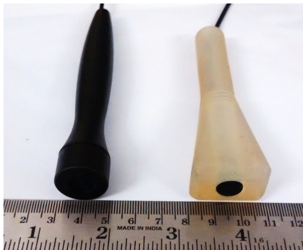
FIGURE 4. Single element ultrasound probes designed for ARTSENS.
