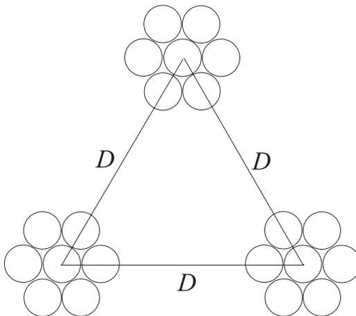
Fig. 5 Line with stranded conductors.
