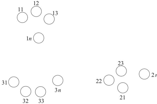
Fig. 2 A three-phase line with composite conductors.
