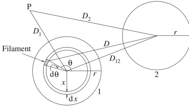
Fig. 1 Cross-section of two parallel straight conductors.
