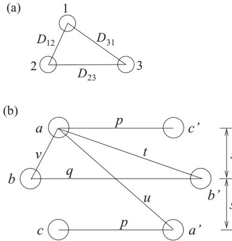
Fig. 3 Single circuit and double circuit lines. (a) Single circuit line; (b) double circuit line.
