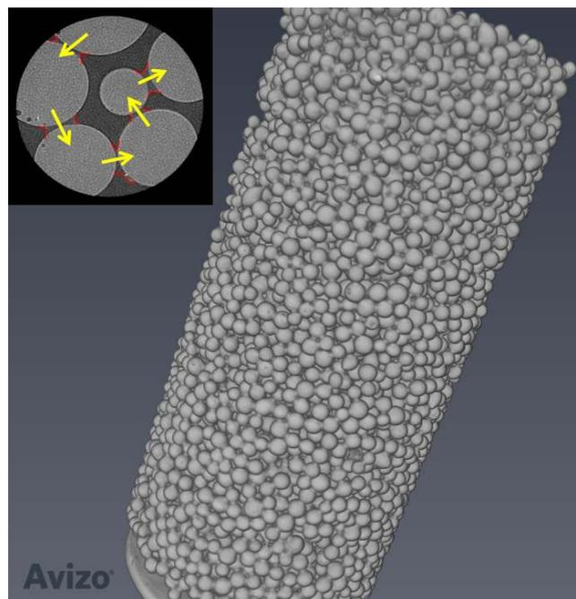
**Figure 1.** Computed tomography image of a weakly cemented specimen (glass ballotini + 1% epoxy) showing a contact bound structure. The inset shows the chain like cemented structure
