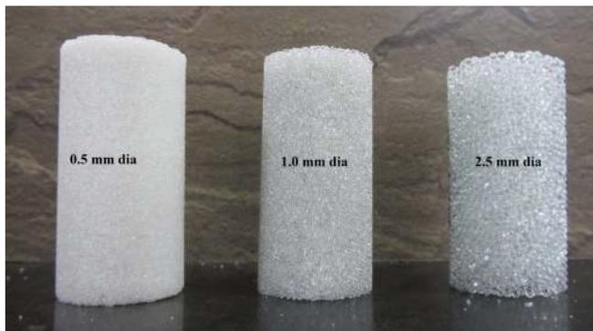
**Figure 3.** Artificially reconstituted weakly cemented (glass balotini + 1% epoxy) specimens with particle size varying from 0.5 to 2.5 mm dia while keeping the system size and density constant
