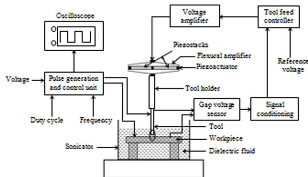
Fig. 1. Schematic diagram of the indigenously developed  $\mu$ -EDM setup
