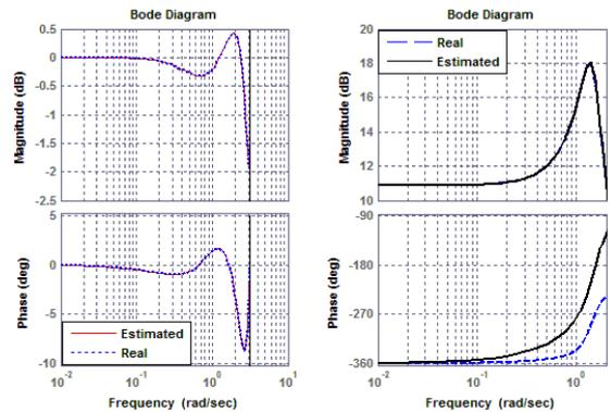
Fig. 8. Bode plots of the closed loop system (left) and plant (right)
