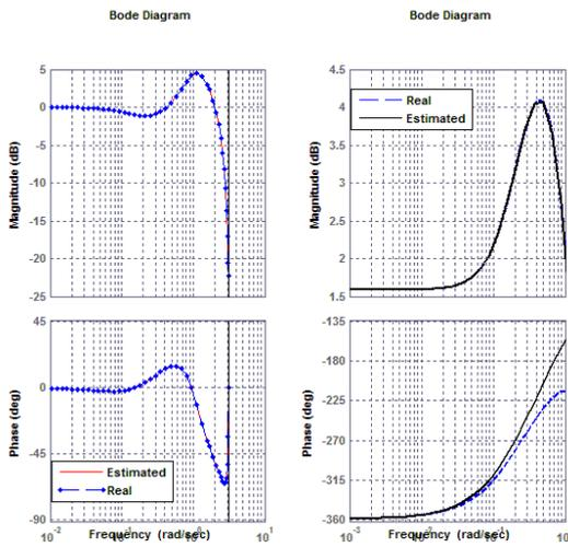
Fig. 5. Bode plots of the closed loop system (left) and plant (right)
