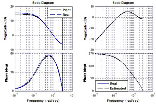
Fig. 2. Bode plots of the plant (left) and closed loop system (right)
