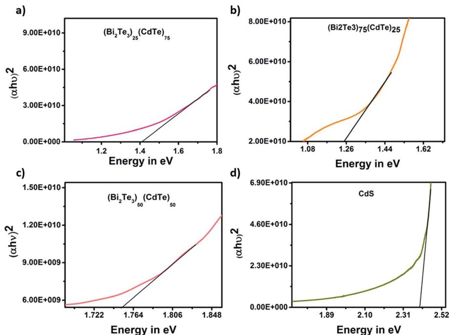
Fig. 8 The energy band gap graph of samples (a)  $(\text{Bi}_2\text{Te}_3)_{25}(\text{CdTe})_{75}$ , (b)  $(\text{Bi}_2\text{Te}_3)_{75}(\text{CdTe})_{25}$ , (c)  $(\text{Bi}_2\text{Te}_3)_{50}(\text{CdTe})_{50}$ , and (d) CdS layer in the fabricated device.
