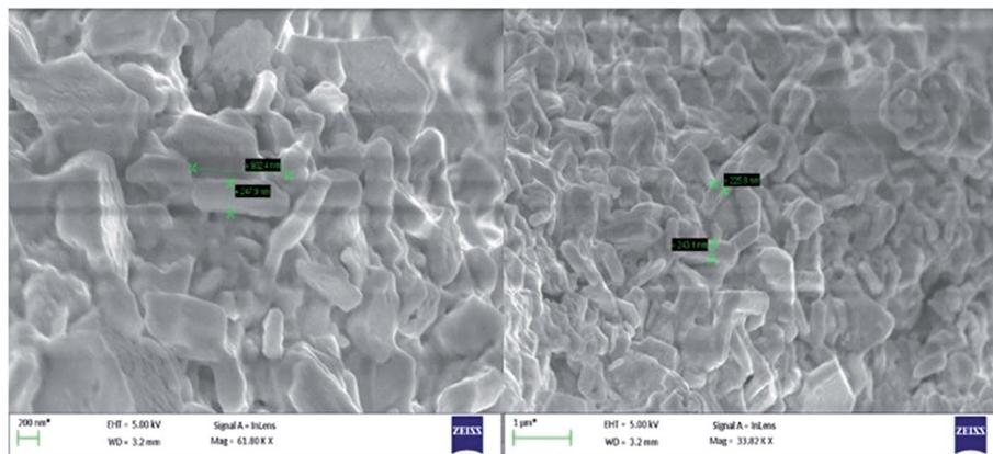
Fig. 5 FESEM morphology of the sample  $(\text{Bi}_2\text{Te}_3)_{25}(\text{CdTe})_{75}$  having nanorods approximately 240 nm in size.
