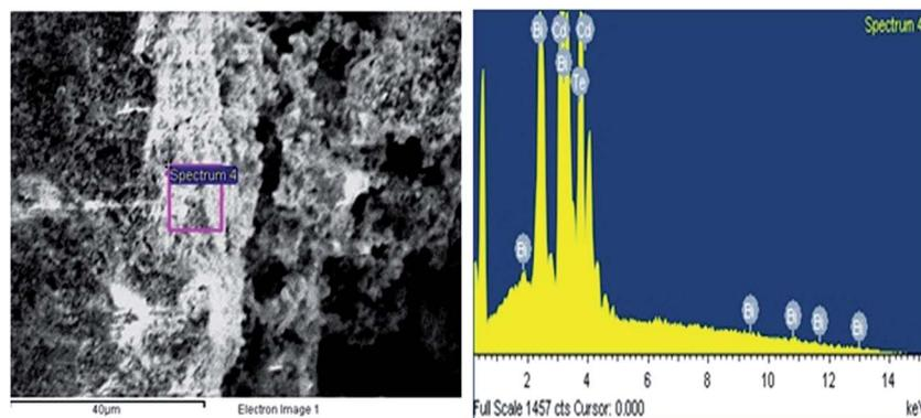
Fig. 6 EDX spectrum of  $(\text{Bi}_2\text{Te}_3)_{25}(\text{CdTe})_{75}$  sample.
