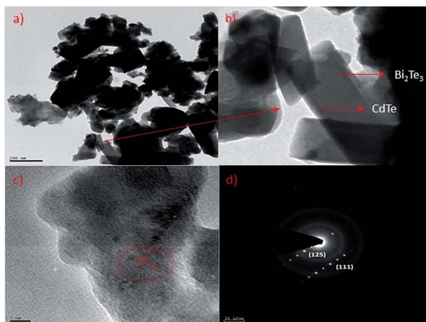
Fig. 3 (a) & (b) Core/shell nanostructure of  $(\text{Bi}_2\text{Te}_3)_{25}(\text{CdTe})_{75}$ ; (c) & (d) electron diffraction (SAED) shows the crystalline structure of  $\text{Bi}_2\text{Te}_3/\text{CdTe}$  in sample  $(\text{Bi}_2\text{Te}_3)_{25}(\text{CdTe})_{75}$ .
