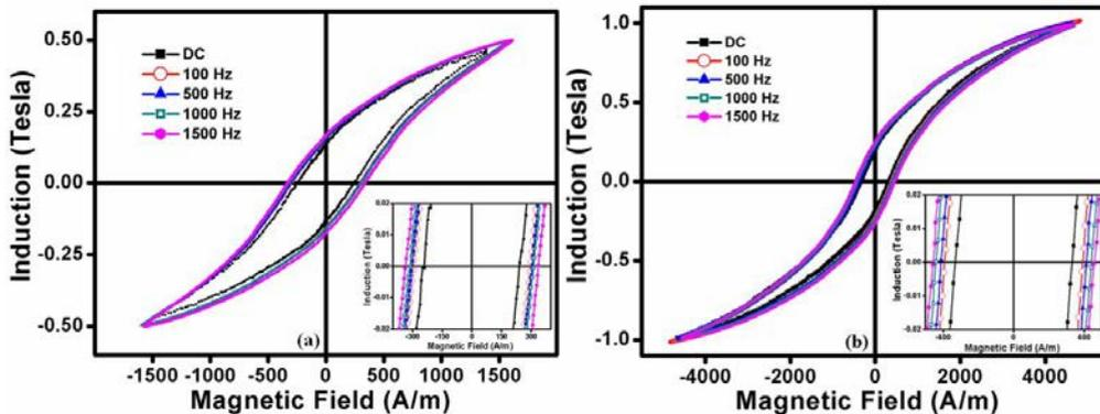
**Figure 5:** DC & AC hysteresis loops of coated iron powder at the induction level of (a) 0.5 Tesla (b) 1 Tesla (colour online).
