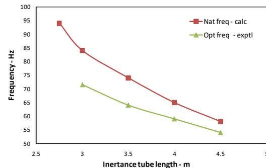
**Figure 8.**  $\phi$  1.76 mm Inertance tube Calculated vs. Optimum Expt. frequency.
