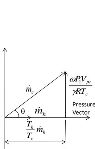
**Figure 2.** Phasor representation for flow through the Pulse tube.
