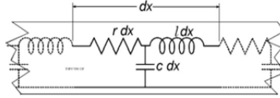
**Figure 4.** Simplified Transmission Line Network [6].
