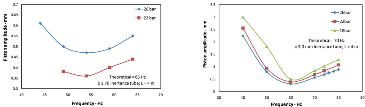
**Figure 11.** Natural frequency experimental data for  $\phi$  1.76 mm and  $\phi$  3 mm Inertance Tubes.
