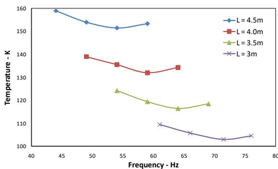
**Figure 7.**  $\phi$  1.76 mm Inertance tube; Temperature variation with Frequency.
