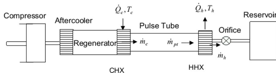
**Figure 1.** Schematic diagram of the Orifice Pulse Tube cryocooler for Phasor analysis.
