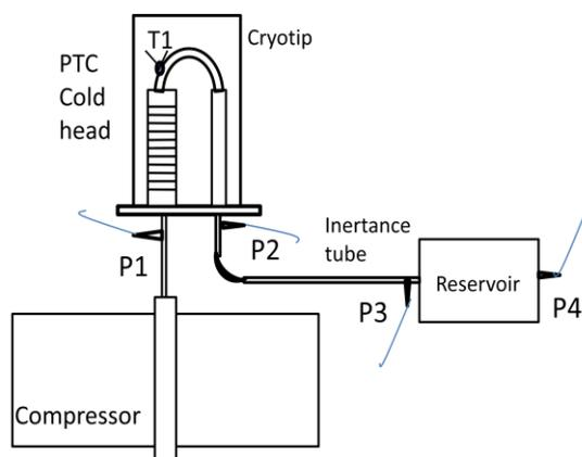
**Figure 5.** Experimental set-up for performance evaluation.
