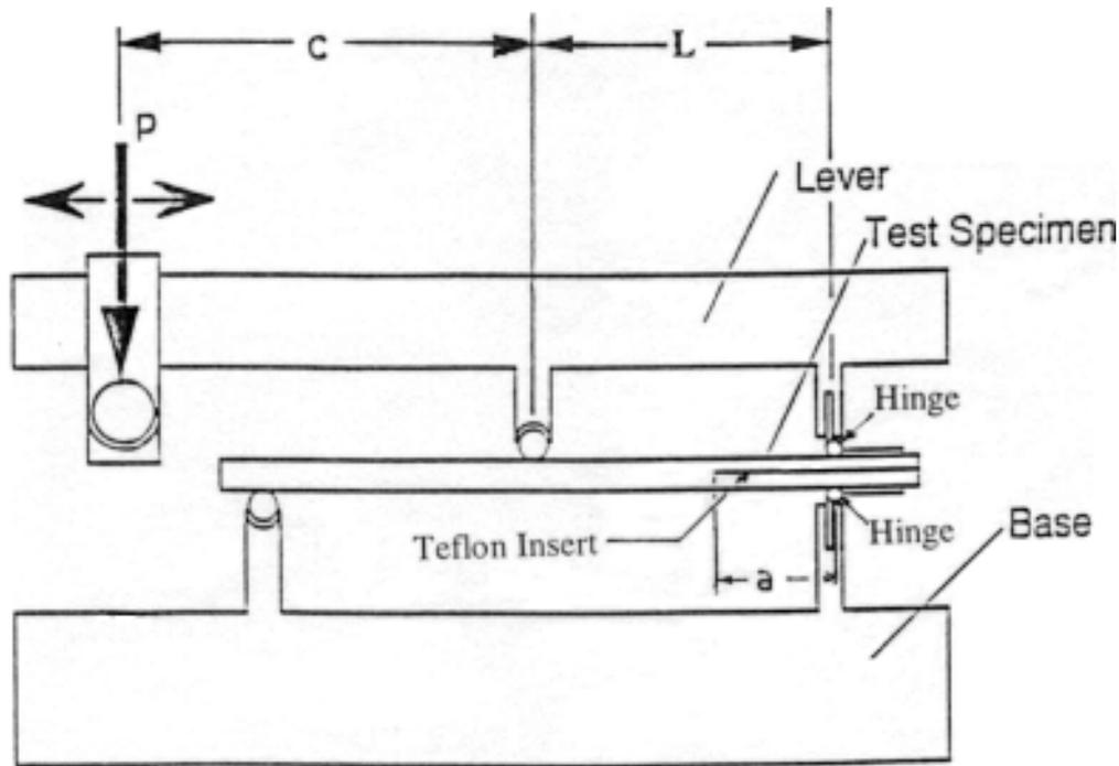
Fig.1. :Schematic Diagram of MMB Specimen and Test Apparatus
