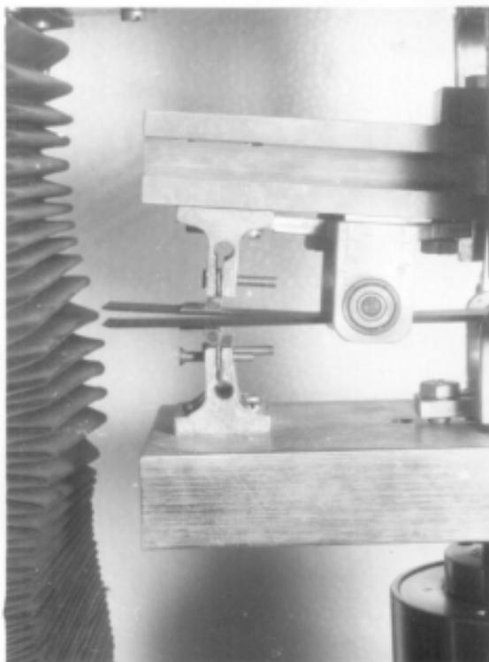
Fig. 2. :MMB Specimen During Testing
