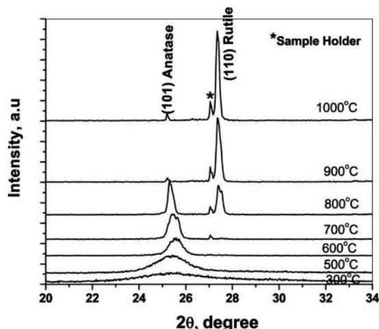
FIG. 7. XRD patterns of  $\text{TiO}_2$  having 5.5 wt % boron at different temperatures.
