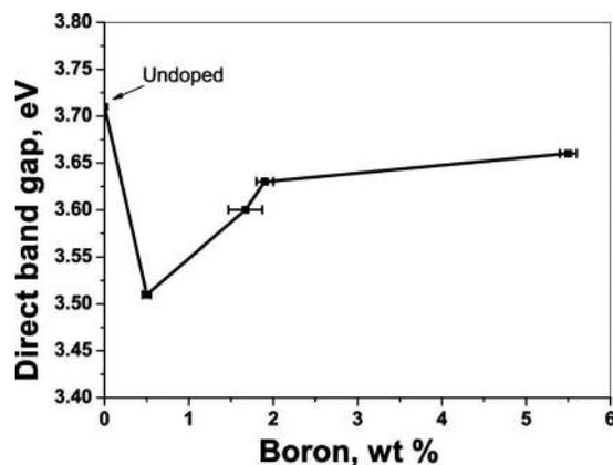
FIG. 13. Change in band gap as a function of boron content.
