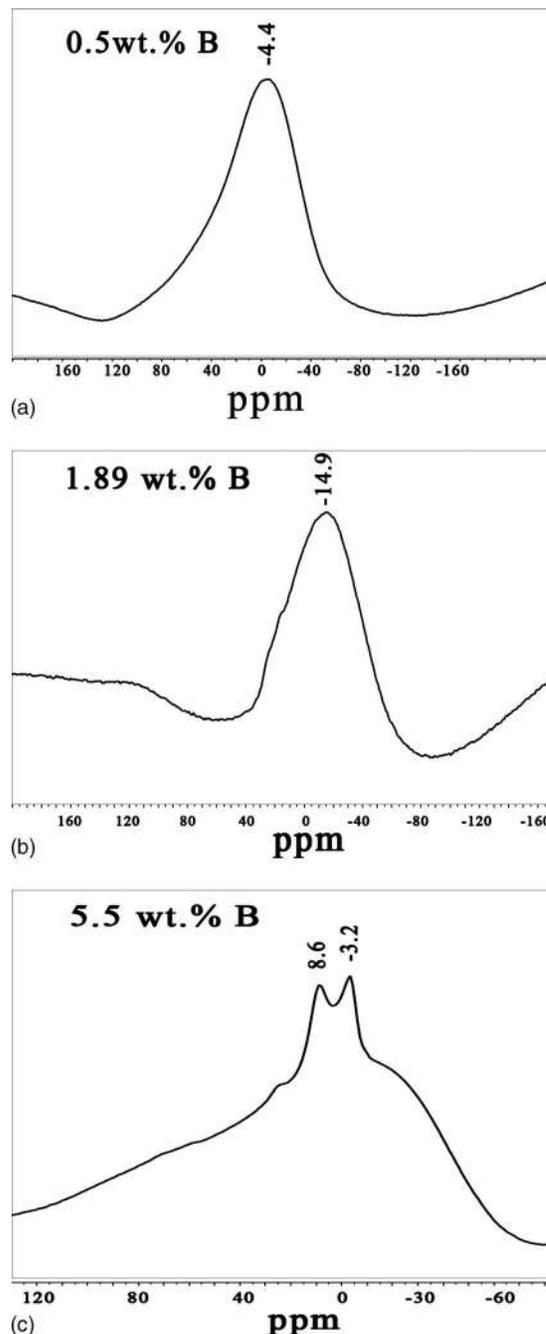
FIG. 4.  $^{11}\text{B}$ -MAS-NMR spectra of B-modified  $\text{TiO}_2$  containing (a) 0.5 wt %, (b) 1.89 wt % B, and (c) 5.5 wt % boron.
