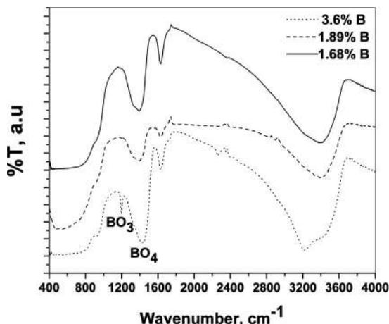
FIG. 5. FTIR spectra of B-modified  $\text{TiO}_2$  for the different synthesized powders.
