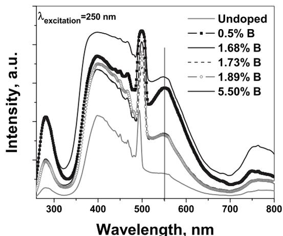
FIG. 14. Emission spectra of the as-synthesized B-modified  $\text{TiO}_2$  at varying boron contents.
