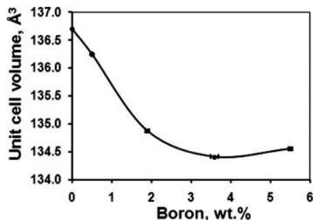
FIG. 11. Change in unit cell volume of anatase with boron content.
