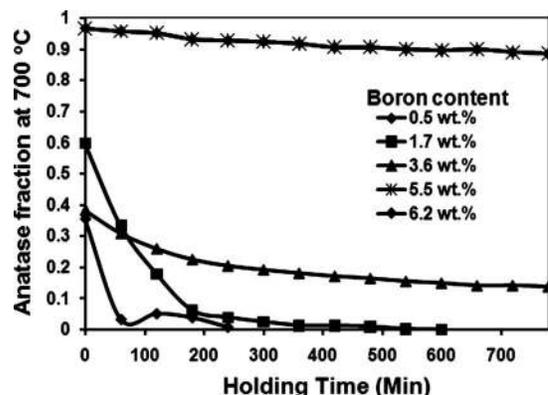
FIG. 9. Change in anatase fraction with time at 700 °C.
