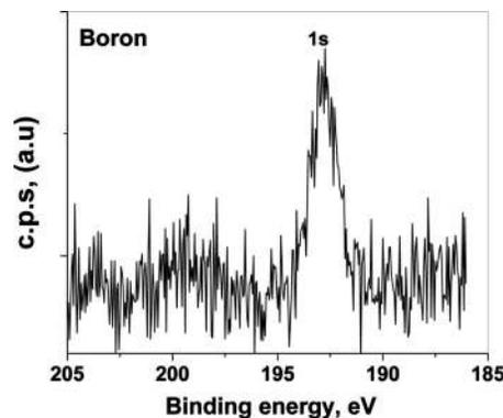
FIG. 2. XPS spectrum of B-modified  $\text{TiO}_2$  having 1.89% boron.
