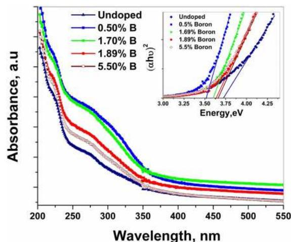
FIG. 12. (Color online) UV-vis spectra of B-modified TiO<sub>2</sub> with varying boron content. The inset gives the  $(ah\nu)^2$ -energy plot.
