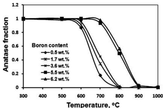
FIG. 8. Change in anatase fraction with temperature.
