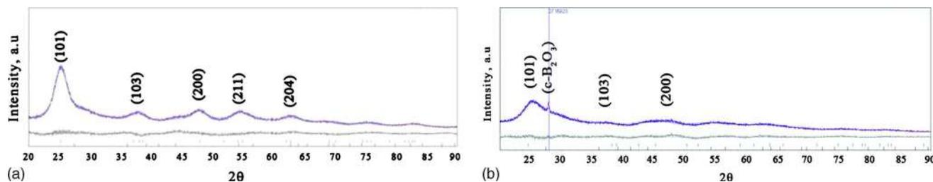
FIG. 1. (Color online) XRD patterns ( $\text{Cu } K\alpha$ ) of the nanocrystalline titania samples having (a) 0.5 wt % boron and (b) 1.89 wt % boron. Presence of cubic  $\text{B}_2\text{O}_3$  was revealed in the XRD pattern of the sample with higher boron content.
