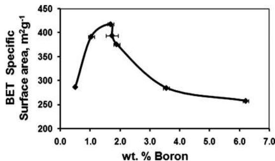
FIG. 6. Specific surface area of B-modified  $\text{TiO}_2$  as a function of boron content.
