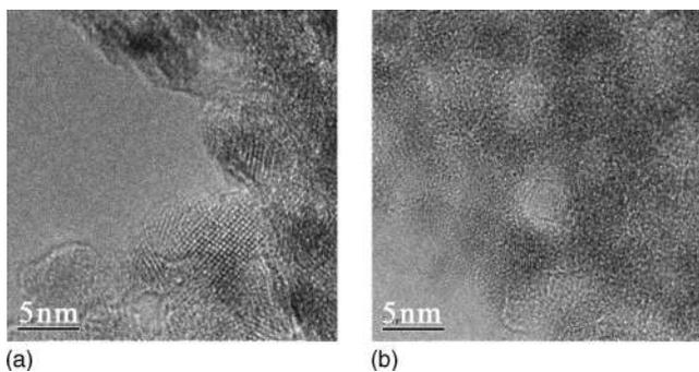
FIG. 3. HRTEM images of samples having (a) 1.7 wt % and (b) 3.6 wt %  $\text{B}_2\text{O}_3$ .
