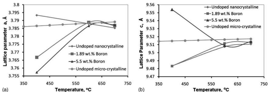
FIG. 10. Effect of boron oxide content on (a) lattice parameter  $a$  and (b) lattice parameter  $c$ , of anatase as a function of temperature.
