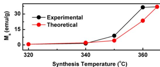
FIG. 5. Saturation magnetization extracted from the room temperature hysteresis loop and calculated theoretically by considering the contribution solely from pure hcp and fcc phases.
