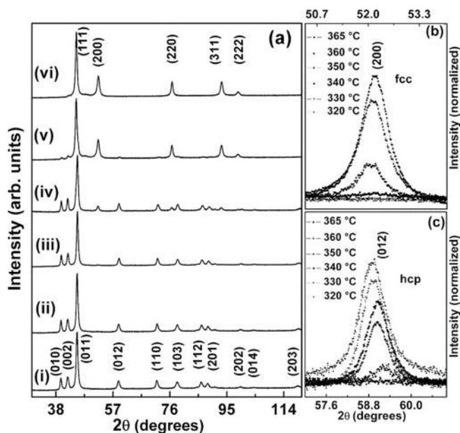
FIG. 1. (a) XRD patterns of nickel nanostructures synthesized at temperatures (i) 320, (ii) 330, (iii) 340, (iv) 350, (v) 360, and (vi) 365 °C, and (b) and (c) show the variation of x-ray intensity of fcc (200) and hcp (012) Bragg's reflections of nickel nanostructures synthesized at different temperatures, respectively.
