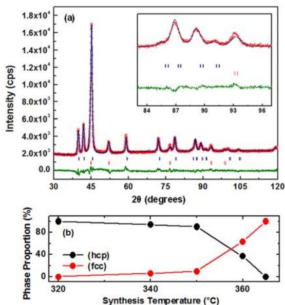
FIG. 2. (a) Measured and simulated (Rietveld method) XRD patterns of nickel nanostructures synthesized at temperature 350 °C and (b) the variation of phase proportion of nickel nanostructures synthesized at different temperatures.
