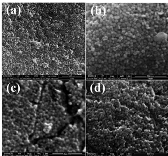
FIG. 3. FESEM images of nickel nanostructures synthesized at temperatures (a) 320, (b) 340, (c) 360, and (d) 365 °C.
