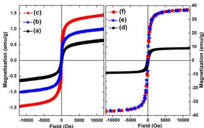
FIG. 4. Field dependent magnetization measured at room temperature of nickel nanostructures synthesized at temperatures (a) 320, (b) 330, (c) 340, (d) 350, (e) 360, and (f) 365 °C.
