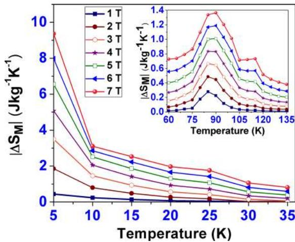
FIG. 4. (Color online) Magnetic entropy change of  $\text{DyMn}_{0.5}\text{Co}_{0.5}\text{O}_3$  from 5 K to 40 K at various magnetic fields. The inset shows magnetic entropy change of  $\text{DyMn}_{0.5}\text{Co}_{0.5}\text{O}_3$  from 60 K to 140 K at various magnetic fields.
