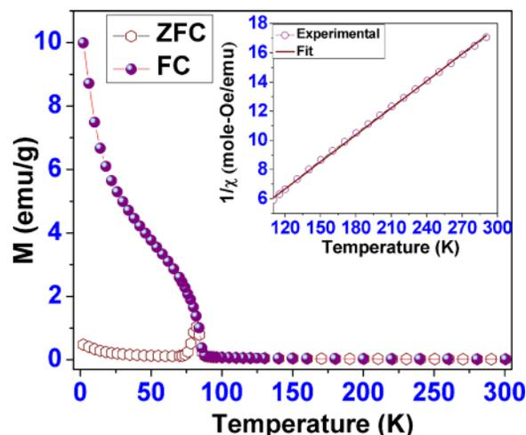
FIG. 1. (Color online) FC and ZFC magnetization vs temperature in an applied field 100 Oe. The inset shows the Curie-Weiss fit.
