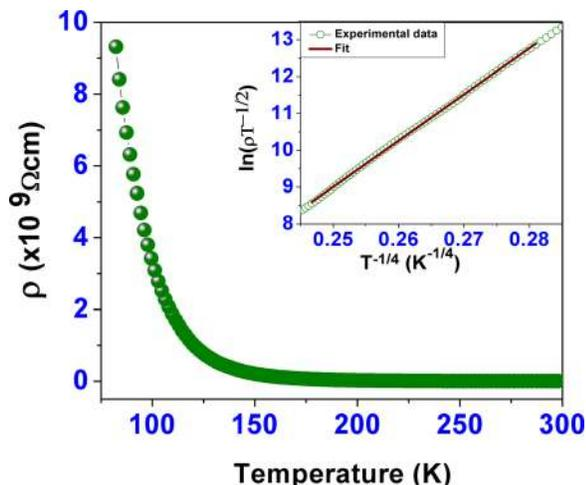
FIG. 5. (Color online) Electrical resistivity vs temperature of  $\text{DyMn}_{0.5}\text{Co}_{0.5}\text{O}_3$ . Inset: VRH model fit.
