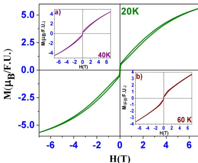
FIG. 3. (Color online) Field dependent magnetization at 20 K. Inset shows field dependent magnetization at (a) 40 K and (b) 60 K.
