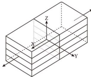
Fig. 5. Laminate geometry and loading
