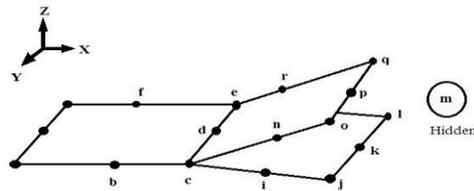
Fig. 2. Illustration of finite element interface nodes near crack front
