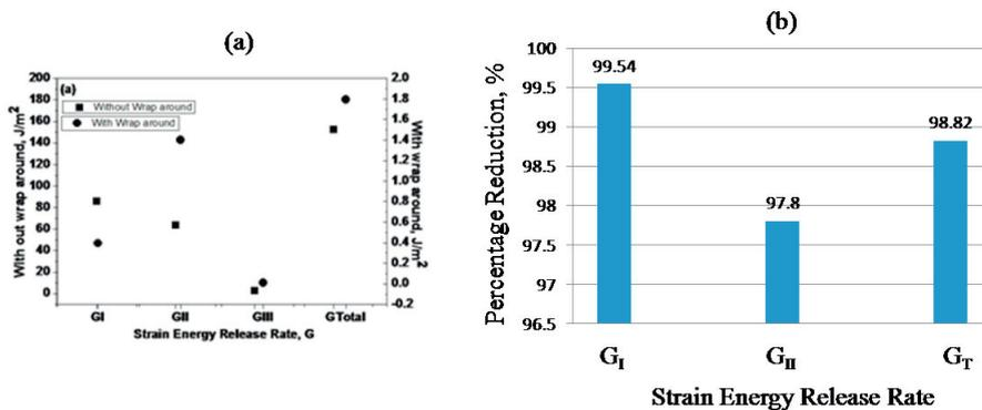
Fig. 11. (a) Strain Energy Release Rate for both models and (b) Percentage of reduction of Strain Energy Release Rate with wrap-around model.
