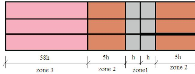
Fig. 6. Zone distribution of one fourth delaminated model
