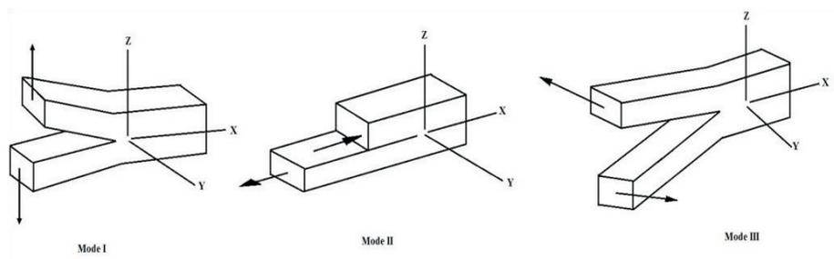
Fig. 1. Basic modes of delamination
