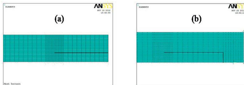
Fig. 7. Finite element representation of (a) without wrap-around laminates and (b) wrap-around laminate
