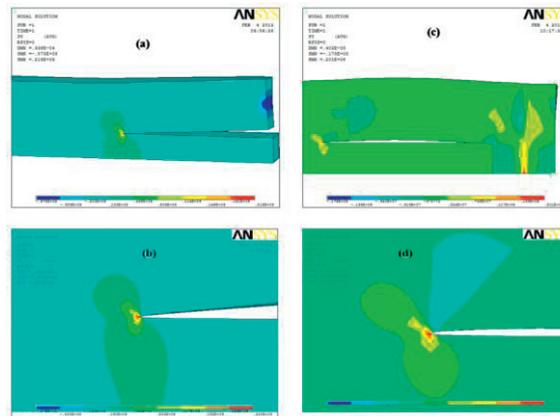
Fig. 8. (a) Contour of inter laminar normal stress distribution in without wrap around model, (b) Enlarged view of normal stress variation around the crack tip (c) Contour of inter laminar normal stress distribution in wrap around model and (d) Enlarged view of normal stress variation around the crack tip
