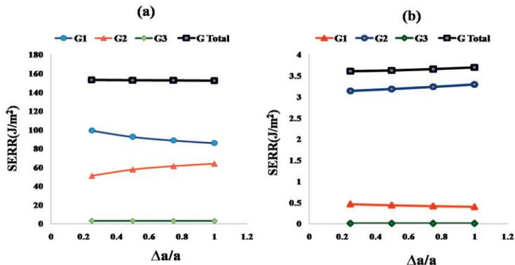
Fig. 10. (a) Convergence study of SEER components of without wrap-around model and (b) Convergence study of SEER components of wrap-around model
