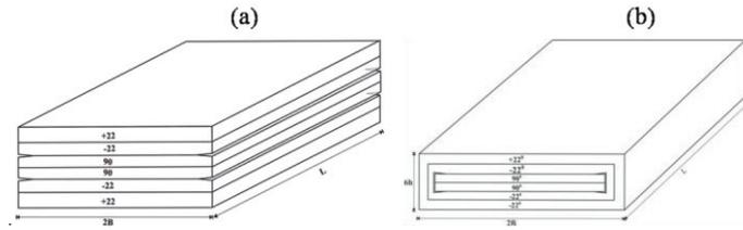
Fig. 3. (a) Delaminated model without wrap-around and (b) Delaminated model with wrap-around
