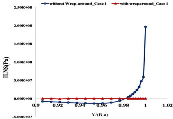
Fig. 9. Distribution of the ILNS ahead of the crack
