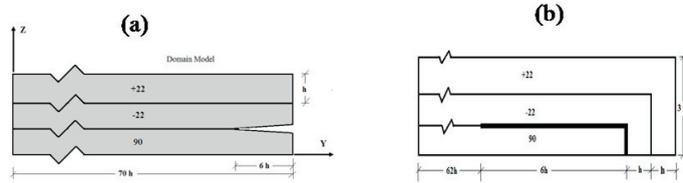
Fig. 4. (a) One fourth model without wrap-around and (b) One fourth model with wrap around
