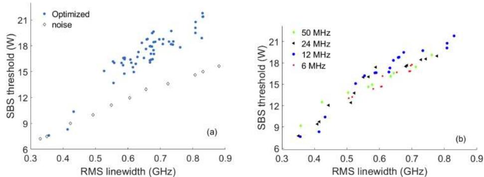
**Fig. 7.** Experimentally measured SBS threshold for optimized waveforms obtained for an amplifier length 10 m at (a) 12 MHz frequency spacing and compared with noise modulation and (b) various frequency spacings.
