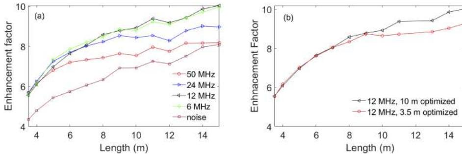
**Fig. 9.** Length dependence of the enhancement factor achieved for (a) optimized waveforms with 650 MHz linewidth obtained for 10 m amplifier at various frequency spacing and their comparison with noise modulation of similar linewidth and (b) optimized waveforms with 650 MHz linewidth obtained for 10 m and 3.5 m amplifier length at 12 MHz frequency spacing
