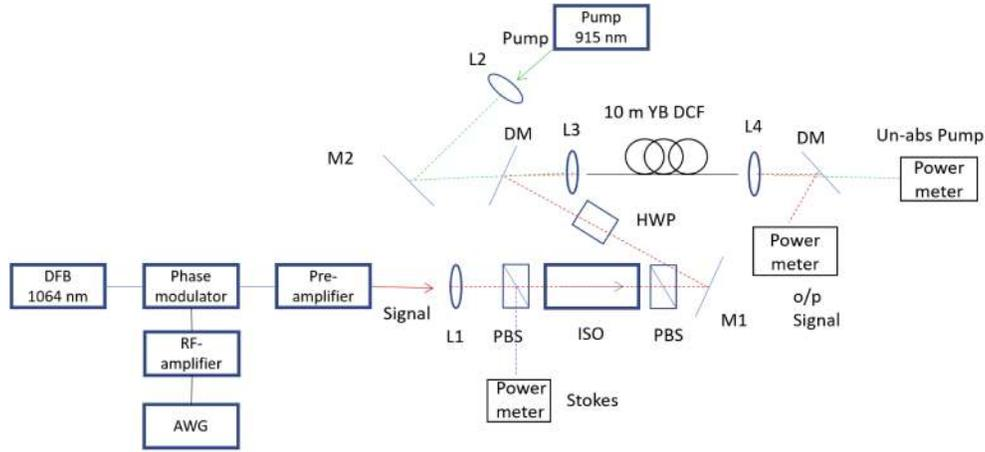
**Fig. 1.** Experimental setup to test the performance of optimized waveforms for suppression of SBS; DFB: distributed feedback laser, PM: power meter, PBS: polarization beam splitter, ISO: Isolator, M: mirror, L:lens, DM: dichroic mirror, HWP: half wave plate, AWG: arbitrary waveform generator.
