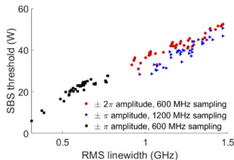
**Fig. 10.** SBS threshold for optimized waveform obtained with higher sampling rate or modulation depth for a 10 m amplifier length and compared with results obtained with lower sampling rate and lower modulation depth
