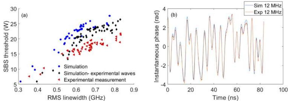
**Fig. 8.** (a) Simulated SBS thresholds with optimized waveforms (blue) and experimentally measured waveforms (black) plotted along with experimentally measured SBS threshold (red) and (b) time trace of a simulated waveform with optical linewidth of 650 MHz to be generated by AWG (blue) and experimental waveform (as recalculated to phase) fed to the phase modulator (red).
