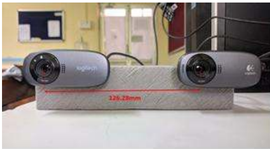
Figure 8. Low-cost stereo camera system
