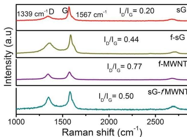
Fig. 4 Raman spectra of sG, f-sG, f-MWNT and sG-f MWNT.
