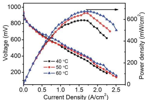
Fig. 8 Polarization graph of Pt/sG-f MWNT (cathode catalyst) and Pt/f-MWNT (anode catalyst) without back pressure.
