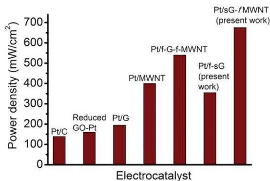
Fig. 9 Comparison of power density obtained with various ORR electrocatalysts.
