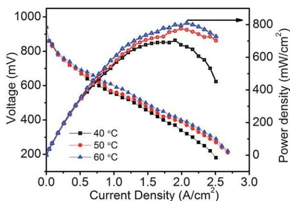
Fig. 10 Polarization graph of Pt/sG-f MWNT (cathode catalyst) and Pt/f-MWNT (anode catalyst) with 1 atm back pressure.
