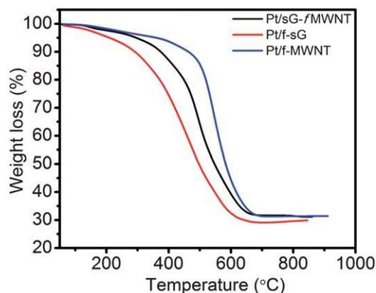
Fig. 5 TGA analysis curves of Pt/f-sG, Pt/f-MWNT and Pt/sG-f MWNT.
