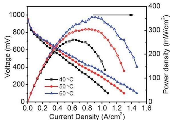
**Fig. 7** Polarization graph of Pt/f-sG (cathode catalyst) and Pt/f-MWNT (anode catalyst).
