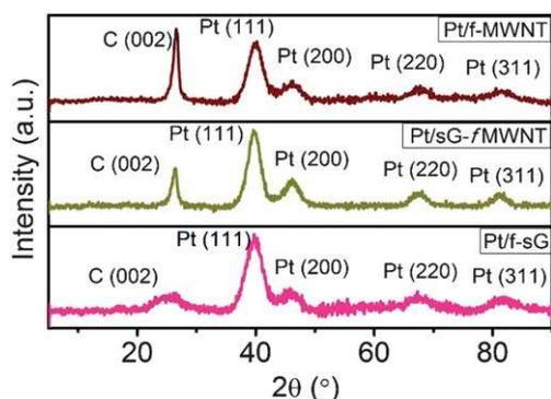
Fig. 3 XRD spectra of Pt/f-MWNT, Pt/sG-f MWNT and Pt/f-sG.
