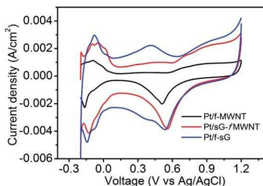
**Fig. 6** Cyclic voltammograms of the electrocatalysts recorded at a scan rate of  $10 \text{ mV s}^{-1}$ . The current normalization has been done with geometric area of the electrode ( $0.07 \text{ cm}^2$ ).
