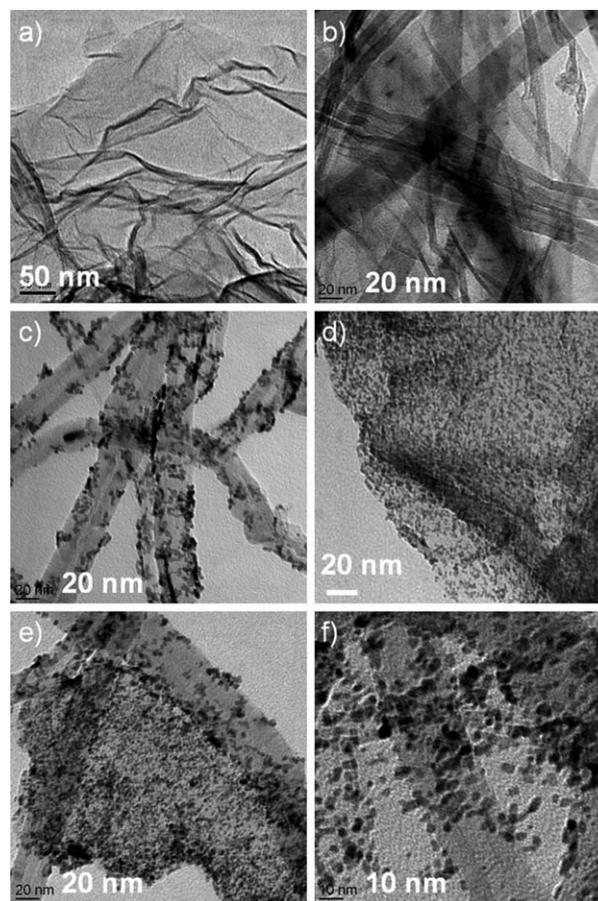
Fig. 2 HRTEM images of (a) f-sG (b) sG-f MWNT (c) Pt/f-MWNT (d) Pt/f-sG (e) low and (f) high magnification images of Pt/sG-f MWNT composite.
