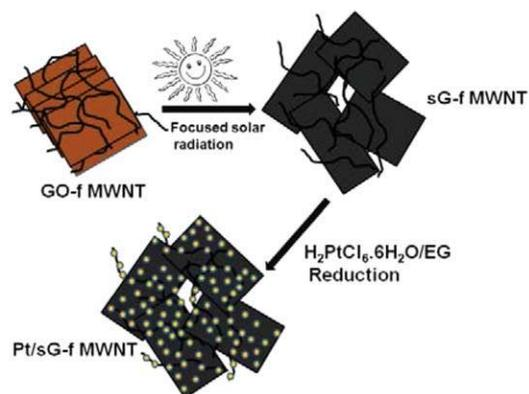
Fig. 1 Schematic for the preparation of Pt/sG-f MWNT.
