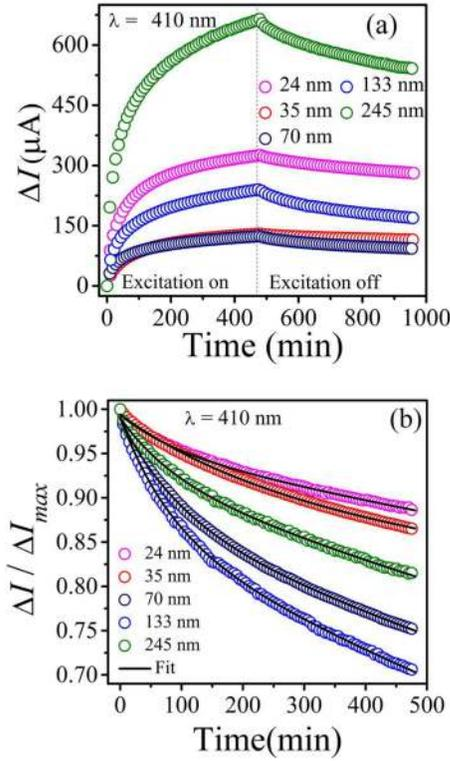
FIG. 2. (a) Change in photocurrent ( $\Delta I$ ) with time under 410 nm illumination for IO films with different thicknesses. The excitation source is switched off after 8 h of illumination. (b) Decay of normalized photocurrent ( $\Delta I/\Delta I_{max}$ ) for IO films with different thicknesses (24 nm–245 nm) under 410 nm illumination.
