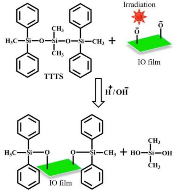
FIG. 6. Schematic representation of surface passivation of IO film through the chemical reaction with TTTs.
