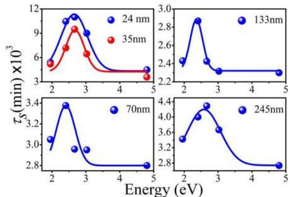
FIG. 7. Variation of  $\tau_s$  with energy of the incident radiation for different film thicknesses. Continuous lines represent the Gaussian fit.
