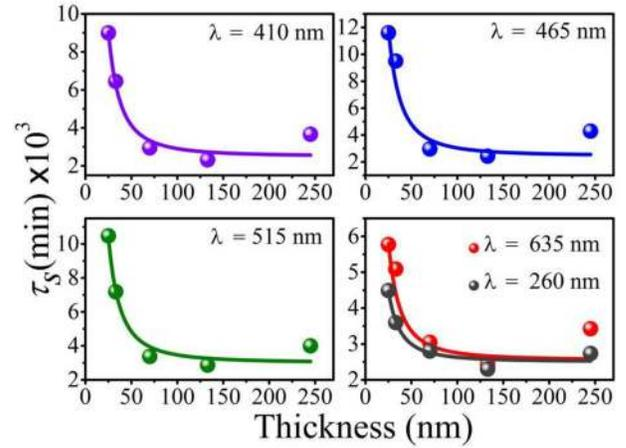
FIG. 3. Thickness dependence of  $\tau_s$  of IO films for different excitation wavelengths (260, 410, 465, 515, and 635 nm). Continuous lines are polynomial fit using Eq. (3).
