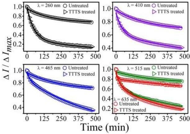
FIG. 5. Decay of normalized photocurrent ( $\Delta I/\Delta I_{max}$ ) of TTTs treated and untreated IO films under different excitations. The thickness of the film is 133 nm. Continuous lines represent the bi-exponential fit.
