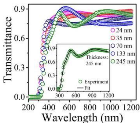
FIG. 1. Optical transmittance spectra of IO films with different thicknesses (24 nm–245 nm). The inset shows transmittance spectra together with theoretical fit (continuous line through data points) for a 245 nm thick film.
