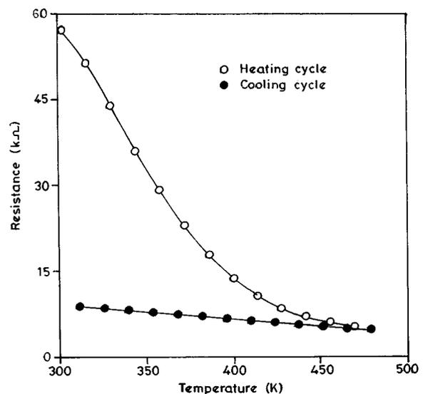
FIG. 3. Variation of resistance with temperature of a typical thin film during heating and cooling cycle.
