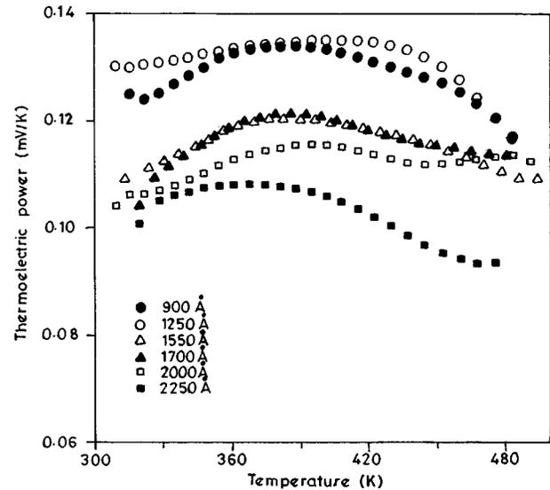
FIG. 5. Variation of thermoelectric power with temperature for thin films of different thicknesses.
