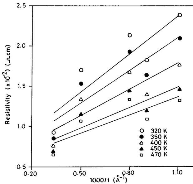
FIG. 6. Plot of resistivity vs reciprocal thickness at different temperatures.
