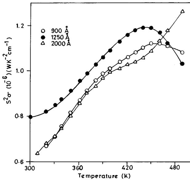
FIG. 8.  $S^2\sigma$  as a function of temperature for different films.
