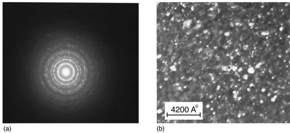
FIG. 2. (a) SAD pattern and (b) electron micrograph of thin film of thickness 1250 Å.
