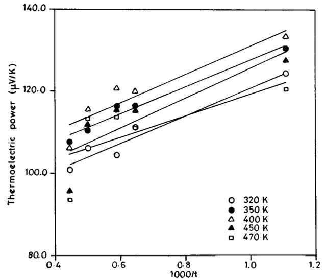
FIG. 7. Plot of thermoelectric power vs reciprocal thickness at different temperatures.
