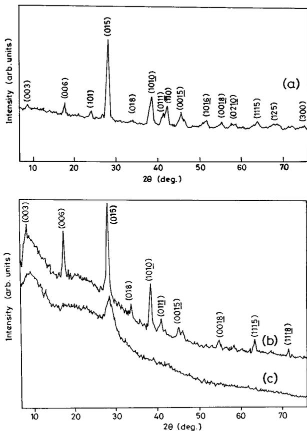
FIG. 1. X-ray diffractogram of  $\text{Bi}_2\text{Te}_2\text{Se}_1$  alloy (a) bulk (b) annealed film (c) unannealed film, film thickness = 2000 Å.
