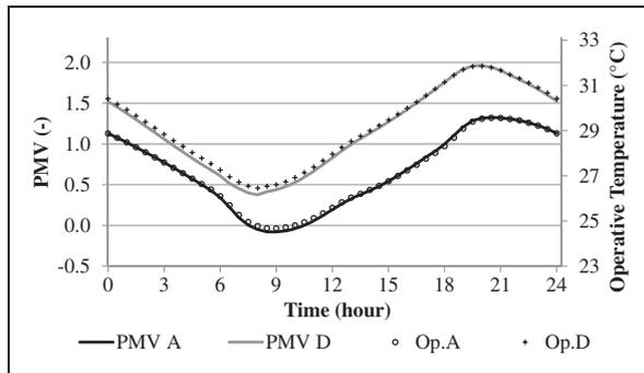
**Figure 14.** Comparison between the PMV and operative temperature (Op.) in Cases A and D of cooling scenario of roof and floor.
