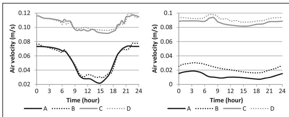
**Figure 10.** The average air velocity in the cooling of the roof and floor (left) and cooling of all surfaces (right) scenarios.
