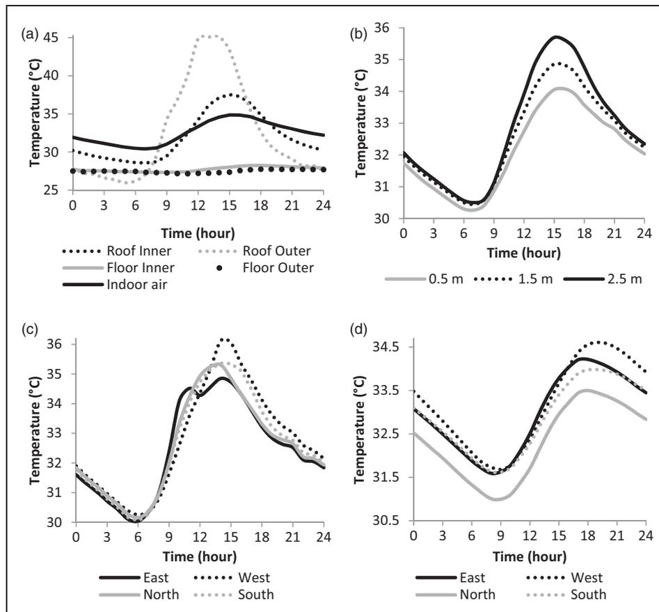
**Figure 6.** Diurnal temperature variation of (a) indoor air, and the roof's and floor's inner and outer surfaces (b) indoor air at various heights (c) outer surface of walls (d) inner surface of walls.
