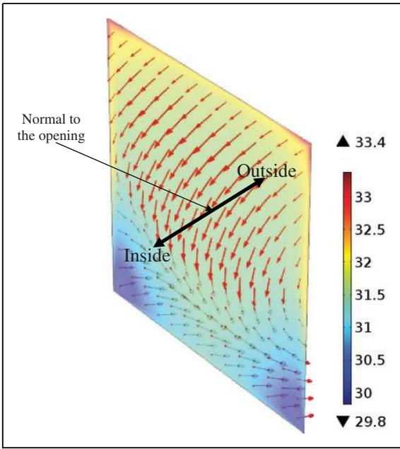
**Figure 11.** Temperature distribution (°C) and velocity arrows at the outlet opening.
