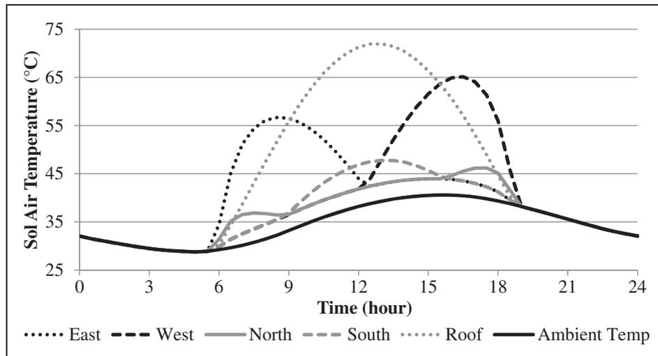
**Figure 4.** Diurnal variation of sol air temperature and temperature of ambient air.
