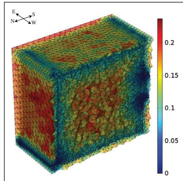
**Figure 5.** Mesh size on cross-section plane facing west direction which was located at the centre of the room.
