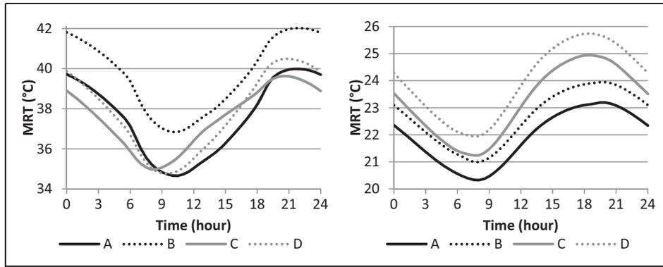
**Figure 9.** Diurnal MRT variation in the no cooling scenario (left) and in the cooling of all surfaces (right).
