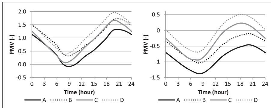
**Figure 13.** PMV in the cooling scenarios of roof and floor (left) and all surfaces (right).
