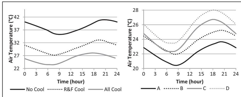
**Figure 8.** The average indoor air temperature in Case D (left) and all surfaces cooling (right).
