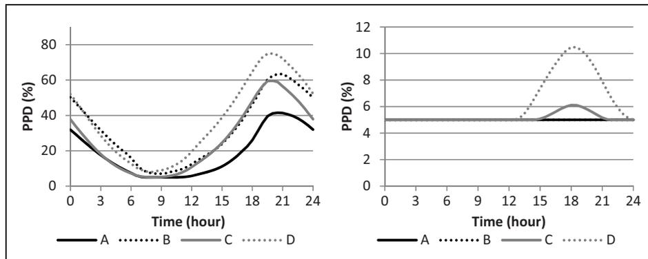
**Figure 15.** The PPD found in the cooling of roof and floor (left) scenario and cooling of all surfaces (right) scenario.
