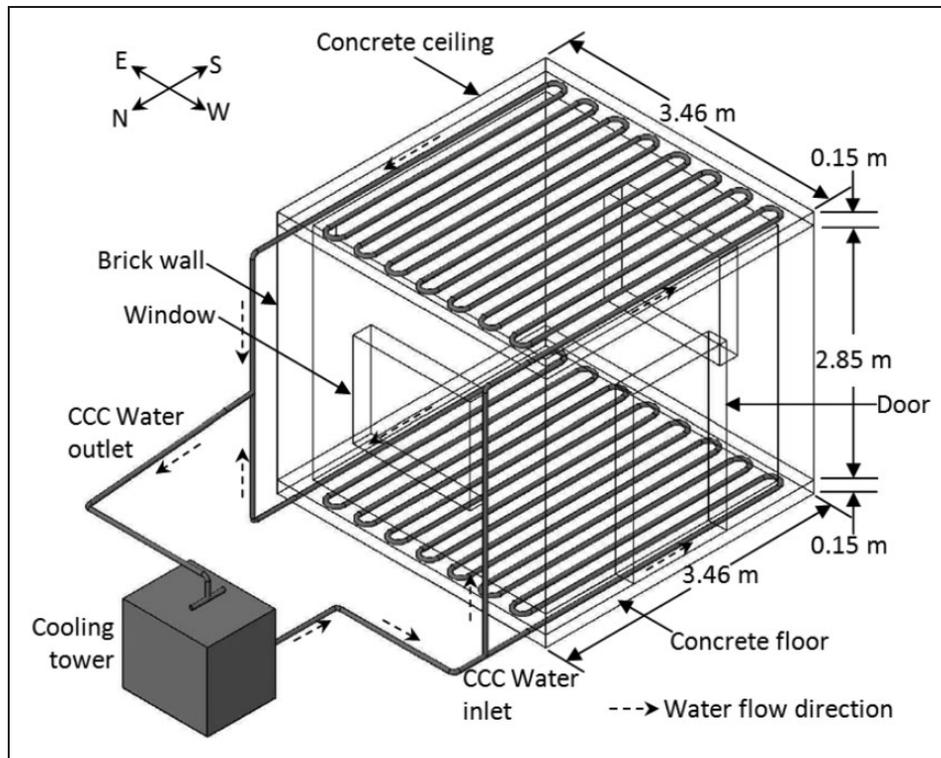
**Figure 2.** Schematic for CCC system supported with cooling tower.
