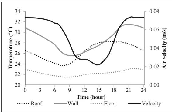
**Figure 12.** The average inner surfaces temperature and average indoor air velocity in the cooling of the roof and floor with no ventilation and no internal load.
