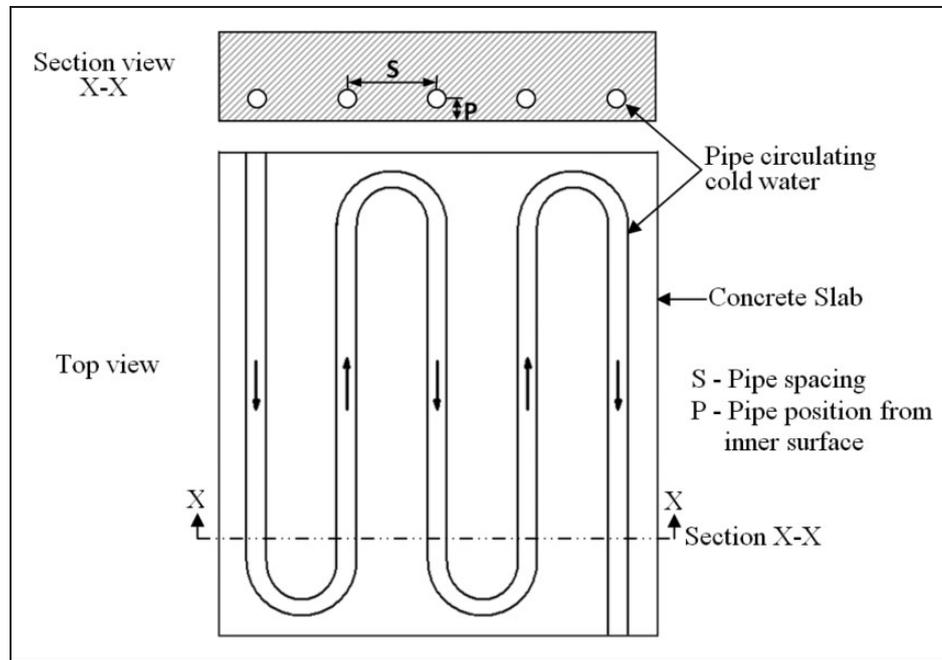
**Figure 1.** Schematic diagram of CCC system.
