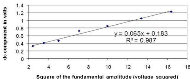
FIG. 3. (Color online) Plot of  $A_{dc}$  with  $A_1^2$  experimentally measured on the AA7175-T7351 sample.
