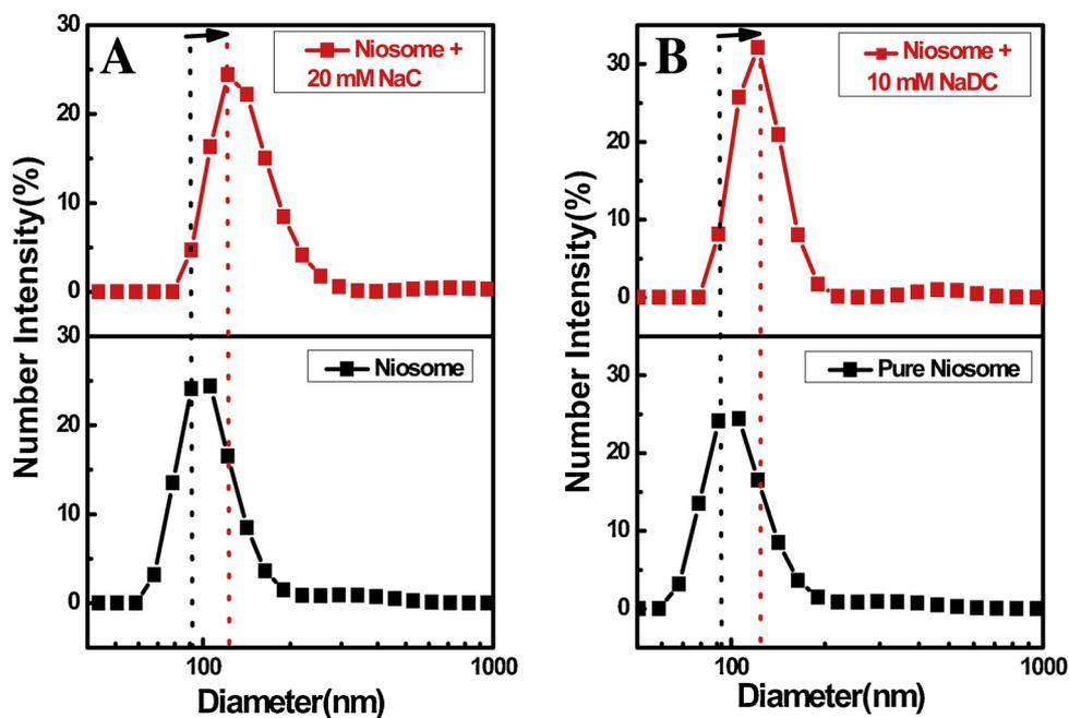
Fig. 1. DLS plot of niosomes in the absence and presence of NaC (A), and NaDC (B) at room temperature, niosomal diameter increases in presence of both NaC and NaDC, [NaC] = 20 mM, [NaDC] = 10 mM.
