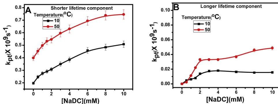
Fig. 7. Variation in the ESPT rate constant ( $k_{pt}$ ) of  $\text{NpOH}^*$  in niosome membrane with increase in NaDC concentration for shorter lifetime component (A) and longer lifetime component (B),  $[1\text{-NpOH}] < 4 \mu\text{M}$ , error =  $\pm 5\%$ .
