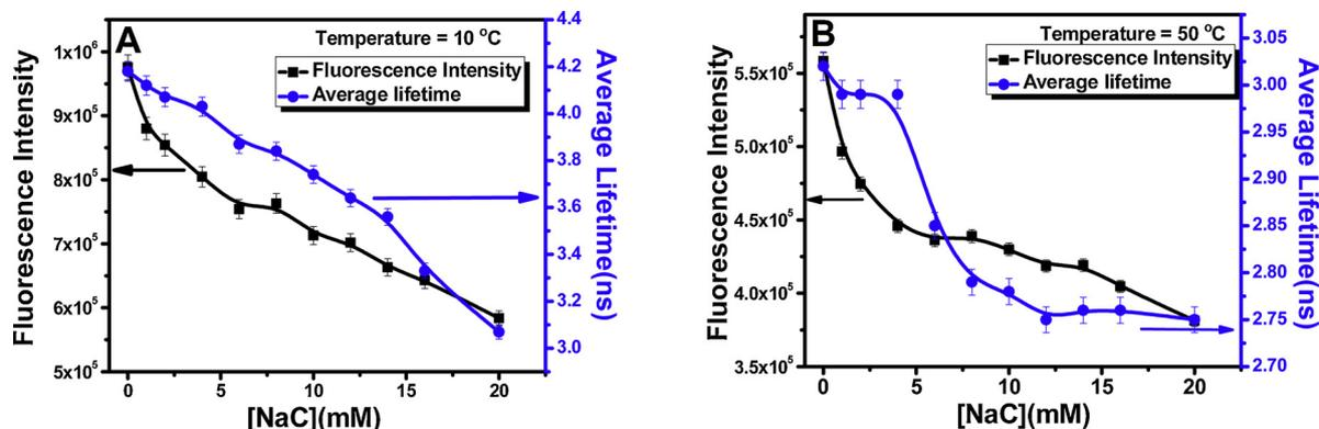
Fig. 4. Variation in steady state fluorescence intensity and average lifetime value of NpOH\* in niosome membrane with variation in NaC concentration at (A) 10 °C, (B) 50 °C,  $\lambda_{ex} = 295$  nm,  $\lambda_{em} = 360$  nm, [1-NpOH] < 4  $\mu$ M, error =  $\pm 5$  %.
