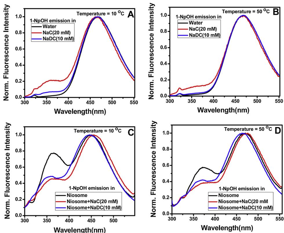
Fig. 2. Normalized emission spectra of 1-NpOH in water and micelle media at (A) 10 °C, (B) 50 °C and in niosomes and niosome-bile salt mixed system at (C) 10 °C, (D) 50 °C, [1-NpOH] < 4 μM, [NaC] = 20 mM, [NaDC] = 10 mM,  $\lambda_{\text{ex}}$  = 290 nm, slit width = 5/5 nm.
