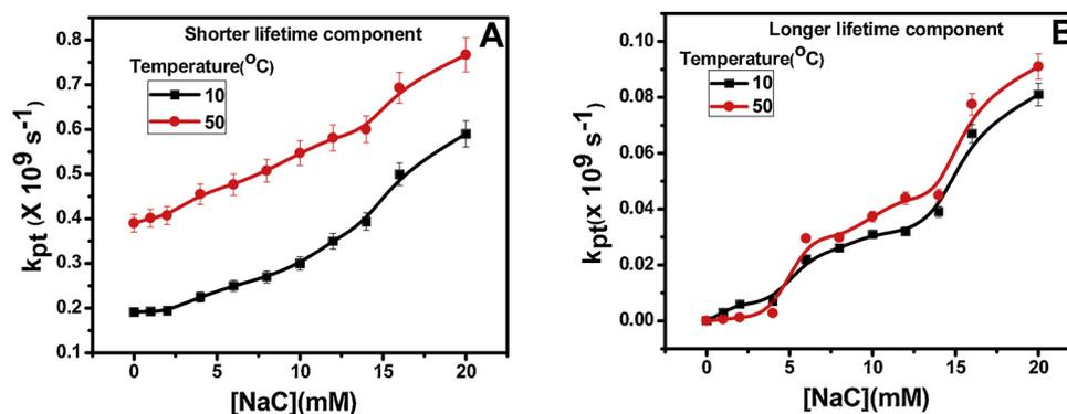
Fig. 5. Variation in ESPT rate constant ( $k_{pt}$ ) of  $\text{NpOH}^*$  in niosome membrane with increase in NaC concentration for shorter lifetime component (A) and longer lifetime component (B),  $[\text{1-NpOH}] < 4 \mu\text{M}$ , error =  $\pm 5\%$ .
