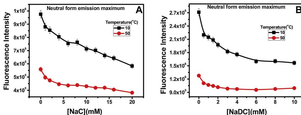
Fig. 3. Point plot of the emission maximum of NpOH\* (360 nm) with increasing NaC (A) and NaDC (B) concentrations at 10 °C and 50 °C,  $\lambda_{ex} = 290$  nm, [1-NpOH] < 4  $\mu$ M, slit width = 5/5 nm, error =  $\pm 3$  %.
