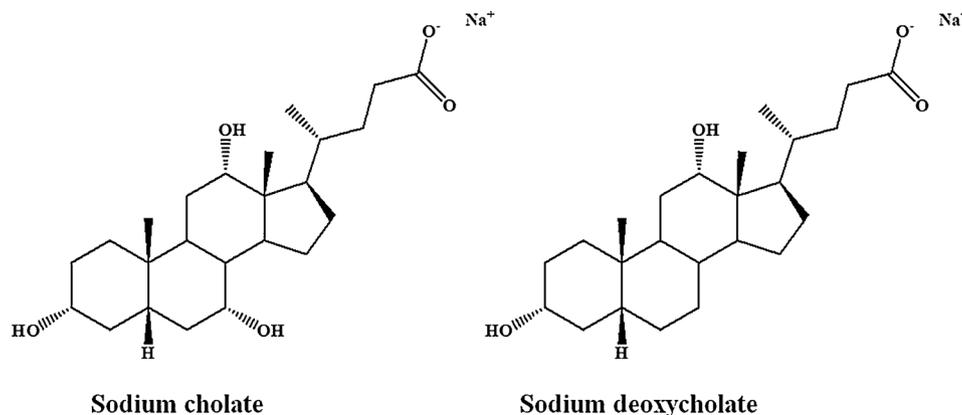
Scheme 1. Chemical structure of (A) sodium cholate (NaC), (B) sodium deoxycholate (NaDC).
