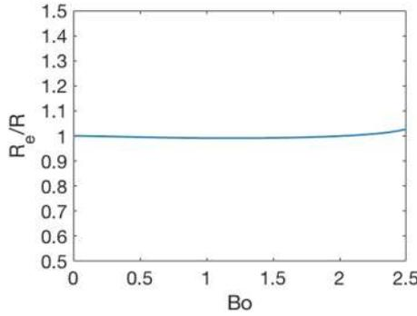
FIG. 6. Variation of the dimensionless equivalent spherical radii with the Bond number based on the bubble cavity radius for the present theory.
