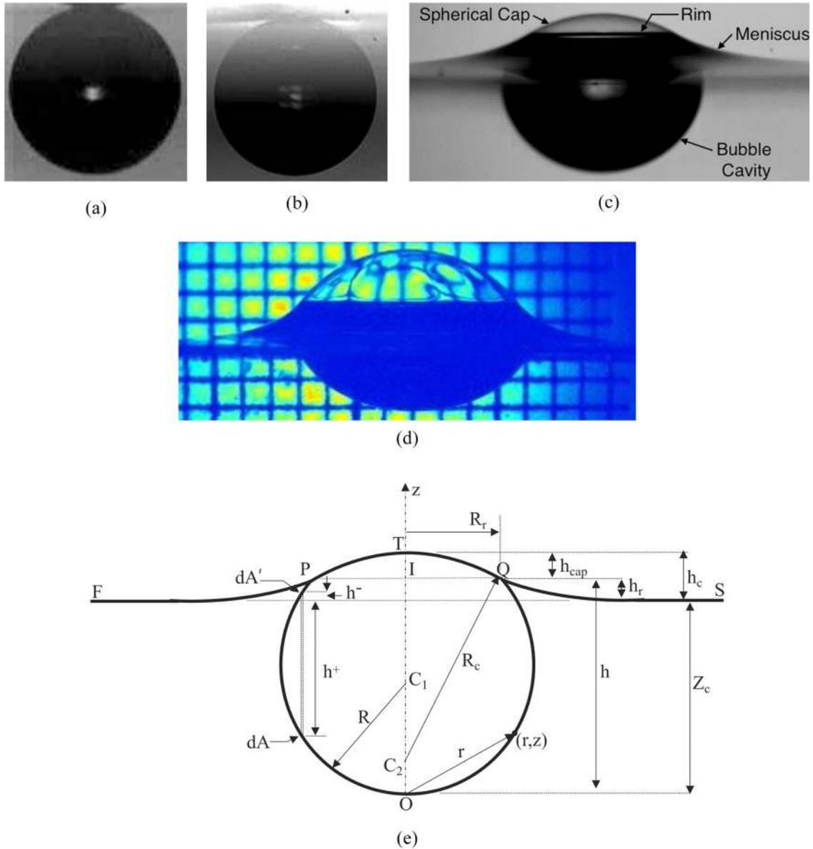
FIG. 1. [(a)–(d)] Side views of floating air bubbles at different Bond numbers. (a)  $R_e = 0.175$  mm,  $Bo_e = 0.004$ ; (b)  $R_e = 0.47$  mm,  $Bo_e = 0.03$ ; (c)  $R_e = 1.99$  mm,  $Bo_e = 0.5$ ; (d)  $R_e = 3.61$  mm,  $Bo_e = 2.46$ ; (e) schematic of a floating bubble with the present notation  $h_c = h_{cap} + h_r$ .
