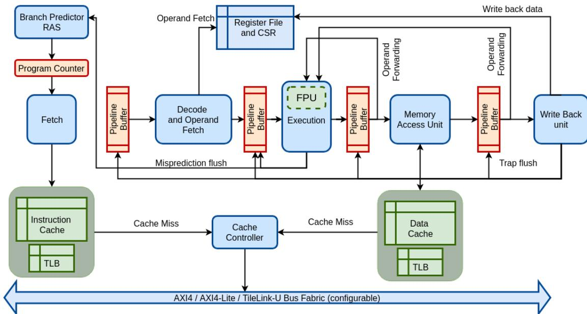
Figure 4: 6-STAGE PIPELINE PROCESSOR DEPICTING MICRO-ARCHITECTURE OF SHAKTI-C
