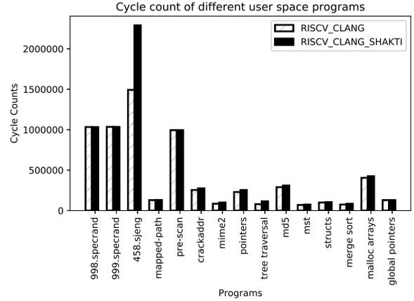
Figure 5: GRAPH DEMONSTRATING CYCLE COUNT OVERHEADS OF DIFFERENT PROGRAMS.
