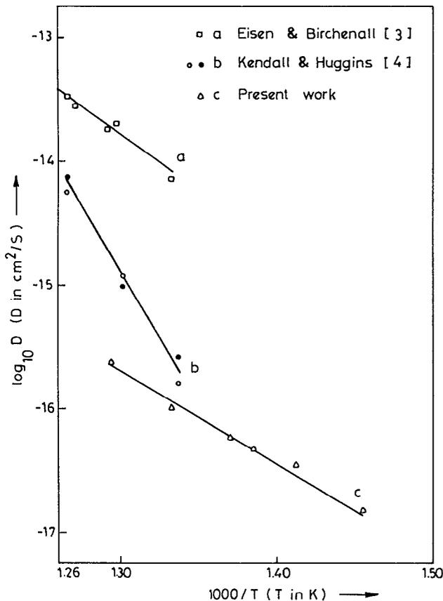
FIG. 7. Comparison of In self-diffusion data of the present work with the previously reported data.
