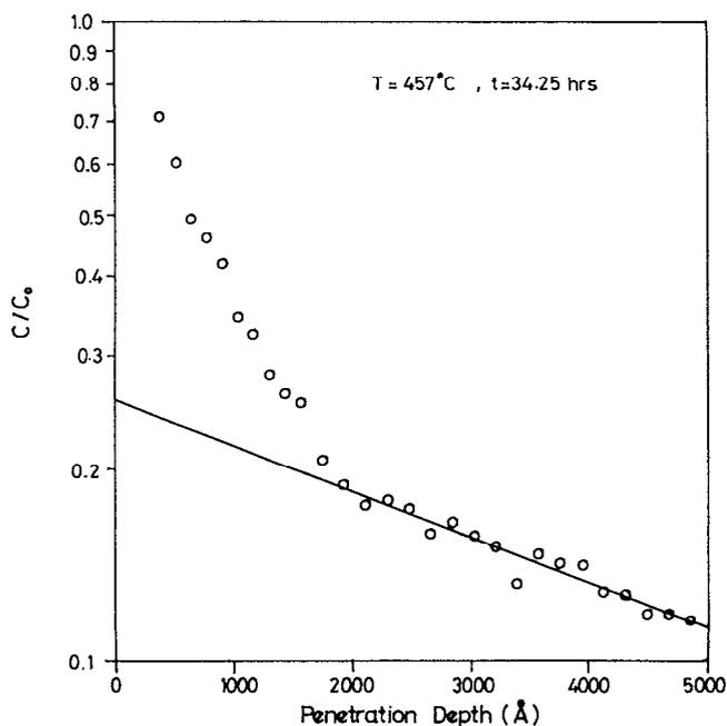
FIG. 3. Relative concentration vs penetration depth for indium diffusion at 457 °C and annealing time 34.25 h. The straight line region represents the dislocation contribution to migration of indium.
