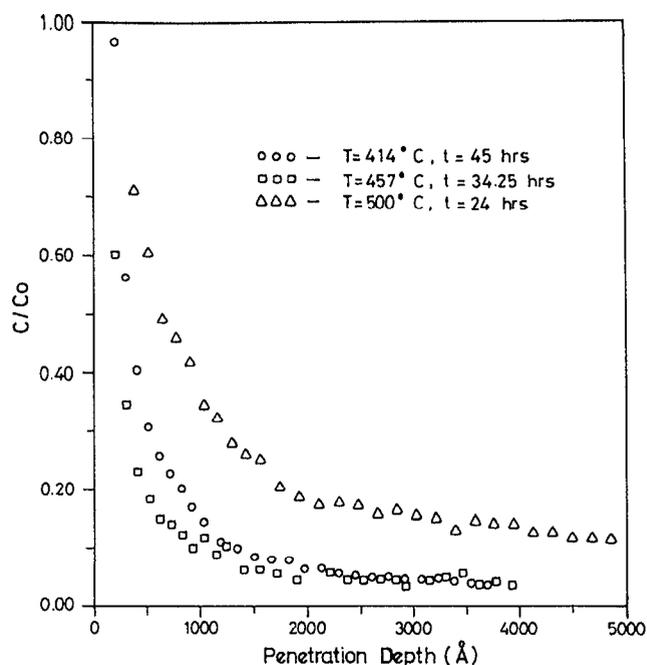
FIG. 1. Representative plots of relative concentration vs penetration depth for indium self-diffusion.
