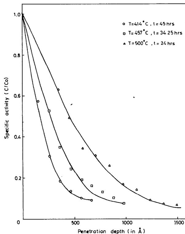
FIG. 4. Indium penetration profiles after subtracting the contribution due to dislocations. Solid lines represent the error function fit.
