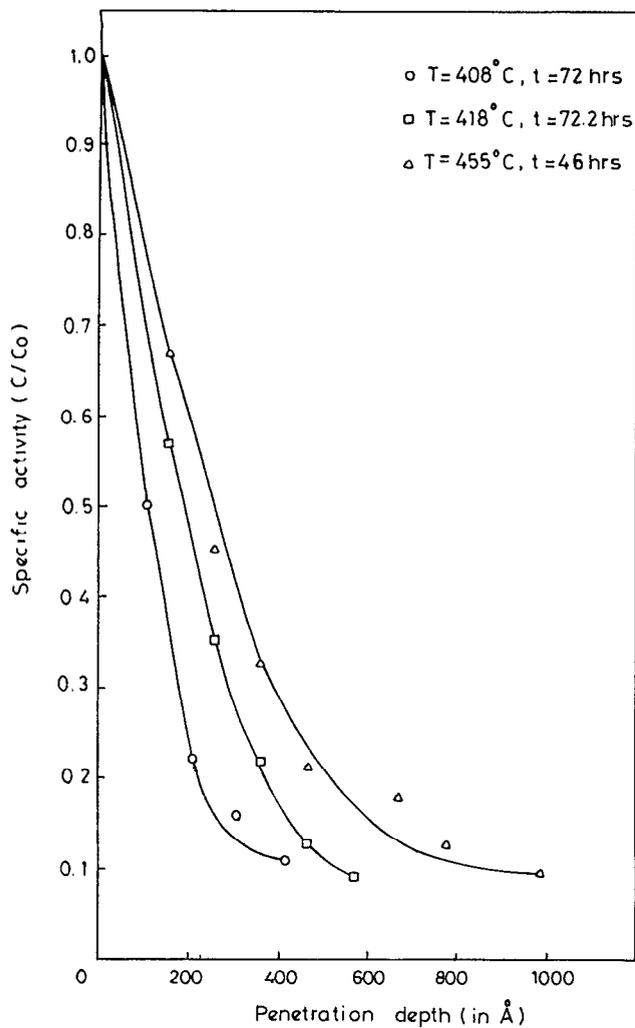
FIG. 5. Antimony penetration profiles after subtracting the contribution due to dislocations. Solid lines represent the error function fit.
