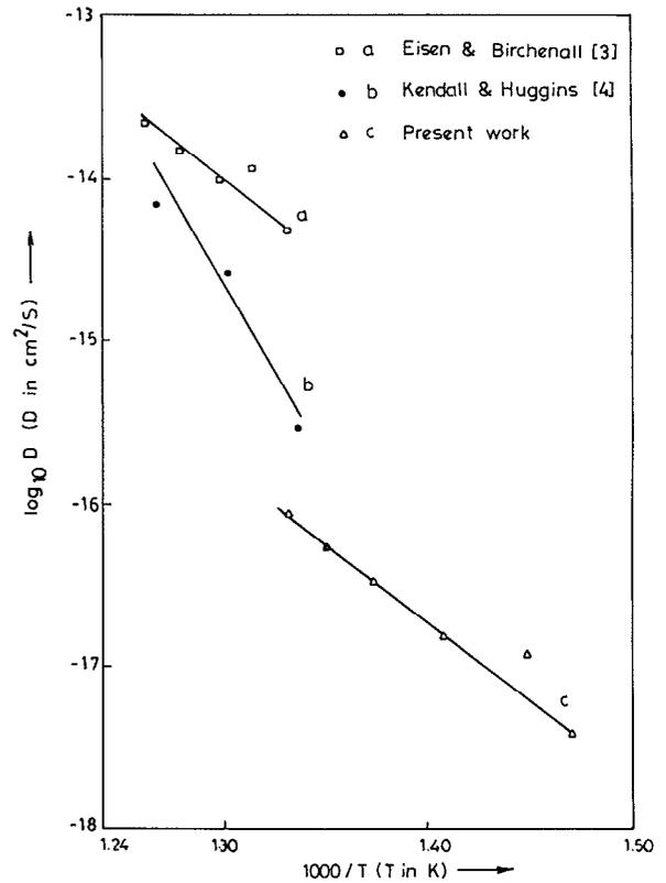
FIG. 8. Comparison of Sb self-diffusion data of the present work with the previously reported data.
