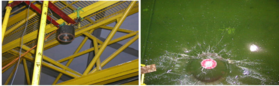
Fig. 6 Electromagnet with protruding strut: (a) Up-close view of the setup for drop test II and (b) WLO touchdown with water surface
