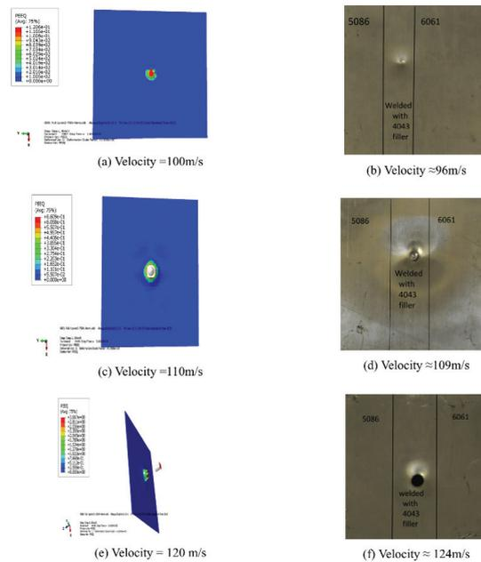
Fig. 4: Complete perforation of Hemispherical bullet on Al plate of 1.2 mm thick Model (a) Velocity = 100m/s; (b) Velocity  $\approx$  96m/s; (c) Velocity = 110m/s; (d) Velocity  $\approx$  109m/s; (e) Velocity = 120 m/s; (f) Velocity  $\approx$  124m/s
