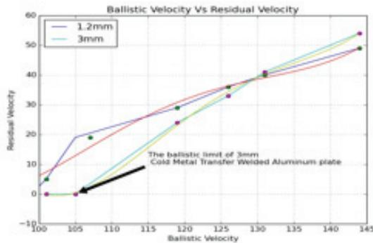
Fig. 5: Ballistic test results conducted on 1.2 mm and 3 mm CMT welded aluminum plates with python coding
