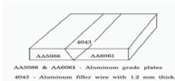
Fig. 1: Layout of weld for joining two dissimilar aluminium grade materials
