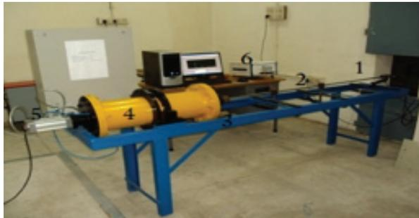
Fig. 3: Layout of laboratory ballistic gun setup comprises of 1.Laser diode, 2.Barrel, 3.Projectile loading point 4.Chamber, 5.Actuator to open the barrel 6.NI data acquisition system
