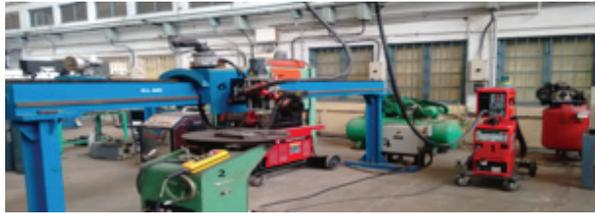
Fig. 2: Layout of welding setup comprises of 1.Digitally controlled MIG/MAG, 2.Power Source, 3.Cooling Unit 4.Robot Control 5.Wire feeder 6.CMT welding torch 7.Wire Buffer
