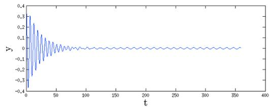
Fig. 9. Structural response under effect of noise at k=100 N/m
