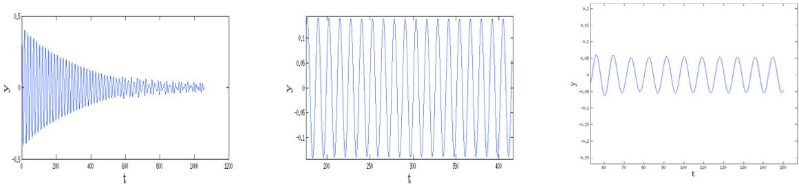
Fig. 7. Deterministic responses at (a) k=15 [pre lock-in] (b) k=30 [lock-in](c) k=80 [post lock-in]
