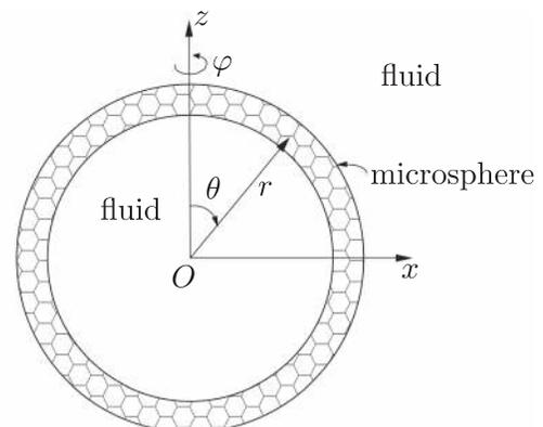
FIG. 1. A thick microspherical shell filled with a fluid and suspended in an other unbounded fluid.
