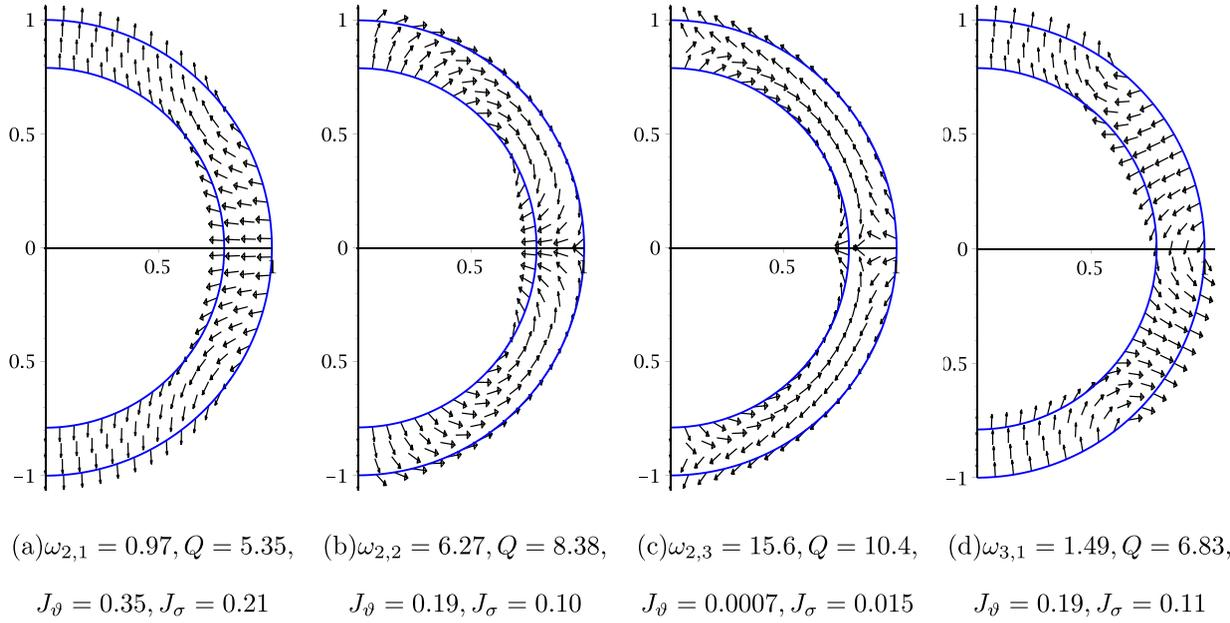
FIG. 4. Vector field plots of different mode shapes for  $n=2$  and  $3$ , and the corresponding eigenfrequencies and deformation measures.
