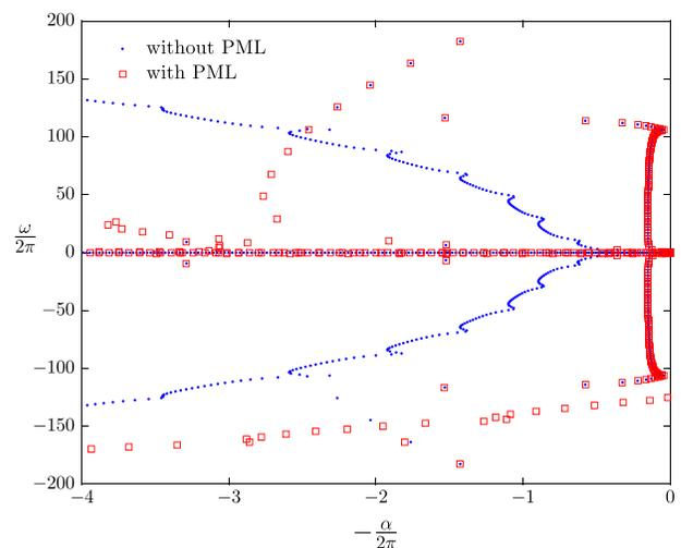
FIG. 7. Eigenspectrum for a meridional wave number  $n=2$  without PML ( $\sigma_0 = 0$ ) and with PML ( $\sigma_0 = 2$ ).
