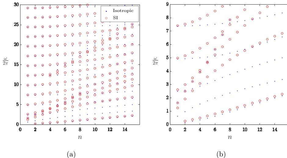
FIG. 3. (a) Variation of eigenfrequency ( $\omega/2\pi$ ) for the meridional wave number from  $n = 1$  to  $n = 15$ , for isotropic and SI material cases. (b) Magnified view of the inset (a) in the low frequency range.
