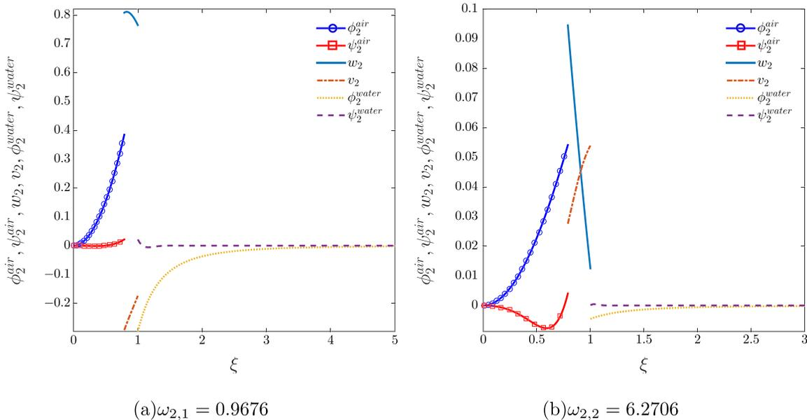
FIG. 5. Variation of radial dependent amplitude functions for the two quadrupole mode shapes and the corresponding responses of air and water along the radial coordinate.
