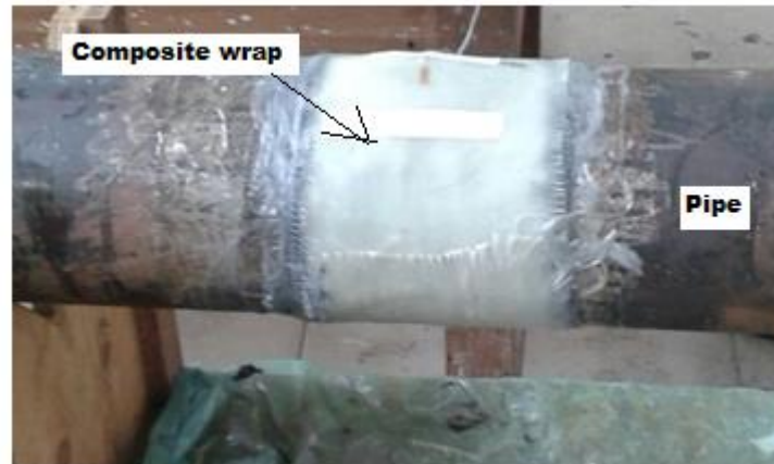
Figure 9. Axial slot defect repaired with elliptical configuration of metallic seal further reinforced with composite sleeve.
