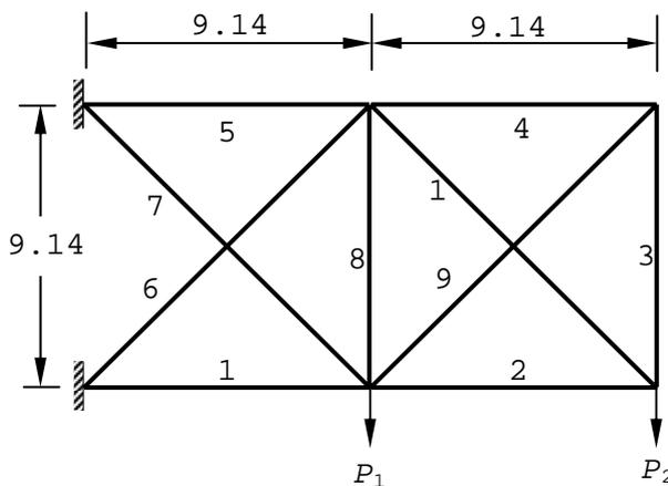
Figure 5. Ten-bar truss (Example 4)
