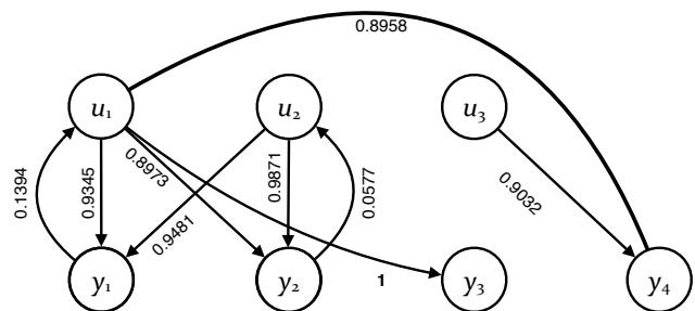
Fig. 4. Connectivity strength for example 3
